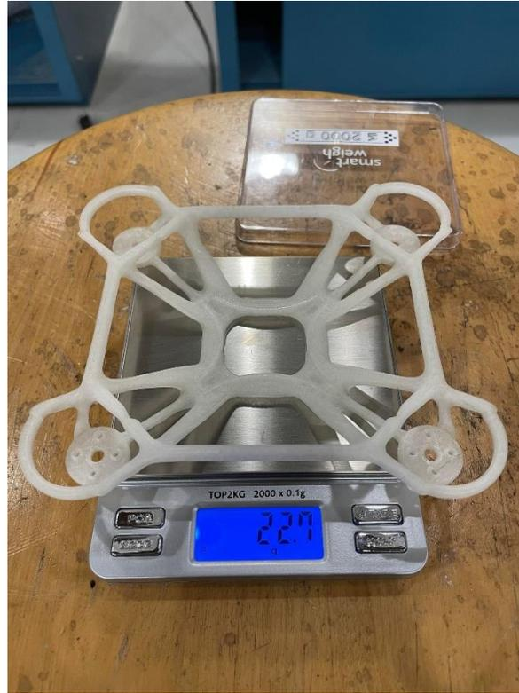
Figure 50: Prototype mass after post-processing.
