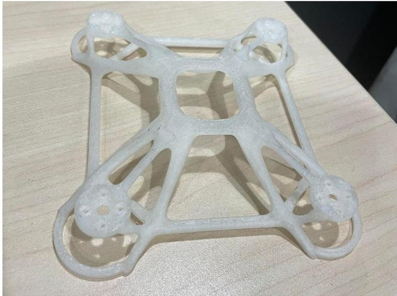
*Figure 42: 3D printed generatively designed outcome 1.*
