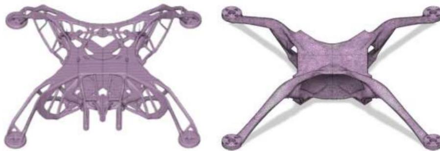
*Figure 8: Generatively designed optimal design outcomes 1 (left) and 2 (right) [4].*
