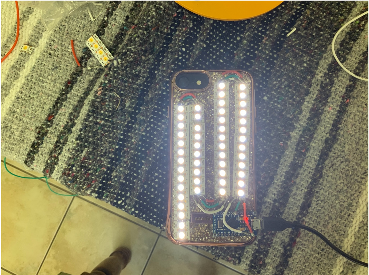
Figure C-2. Images Throughout the Soldering Process. This image portrays the 51 lights soldered together and placed on the back of my phone case to ensure the arrangement fits the surface area.
