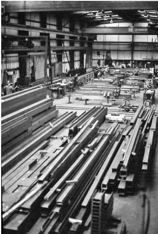
FIGURE 2. Reclaimed steel stored ready for refabrication.
