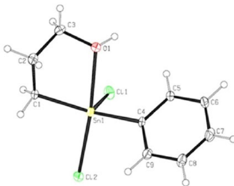
Figure 30. ORTEP representation of 11 found in the unit cell and selected bond lengths [Å] and angles [°]. Thermal ellipsoids drawn at the 30% level. Sn \cdots O 2.400(3), Sn-Cl1 2.3766(14), Sn-Cl2 2.4509(12), Cl1-Sn-Cl2, 94.20(5), C1-Sn-C4 143.79(18), O \cdots Sn-Cl2 173.88(9).
