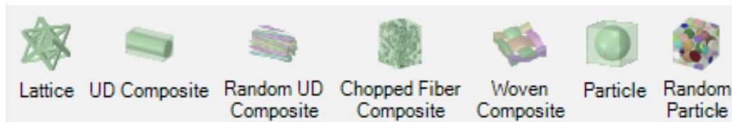
Figure 2-6: Shape of Representative Volume Element in ANSYS [10]
