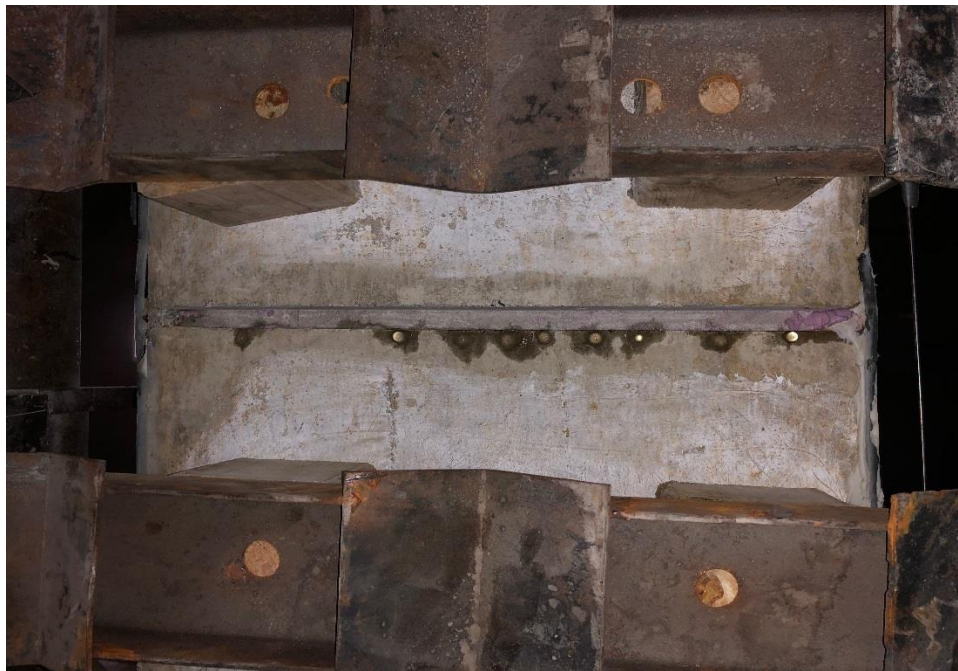
Figure 4-22: Leakage of the NC3 specimen repaired using ECC fly ash under 8 psi water pressure (bottom face)
