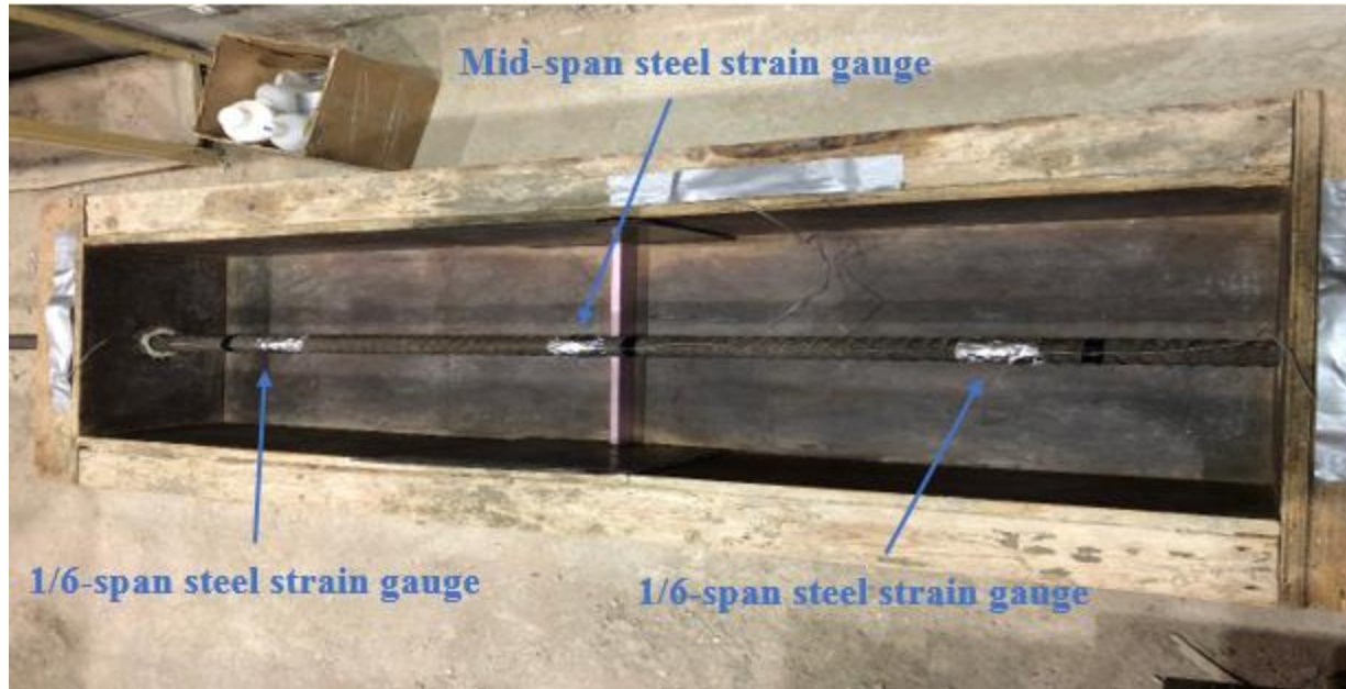
Figure 3-16: Arrangement of steel strain gauges on the rebar
