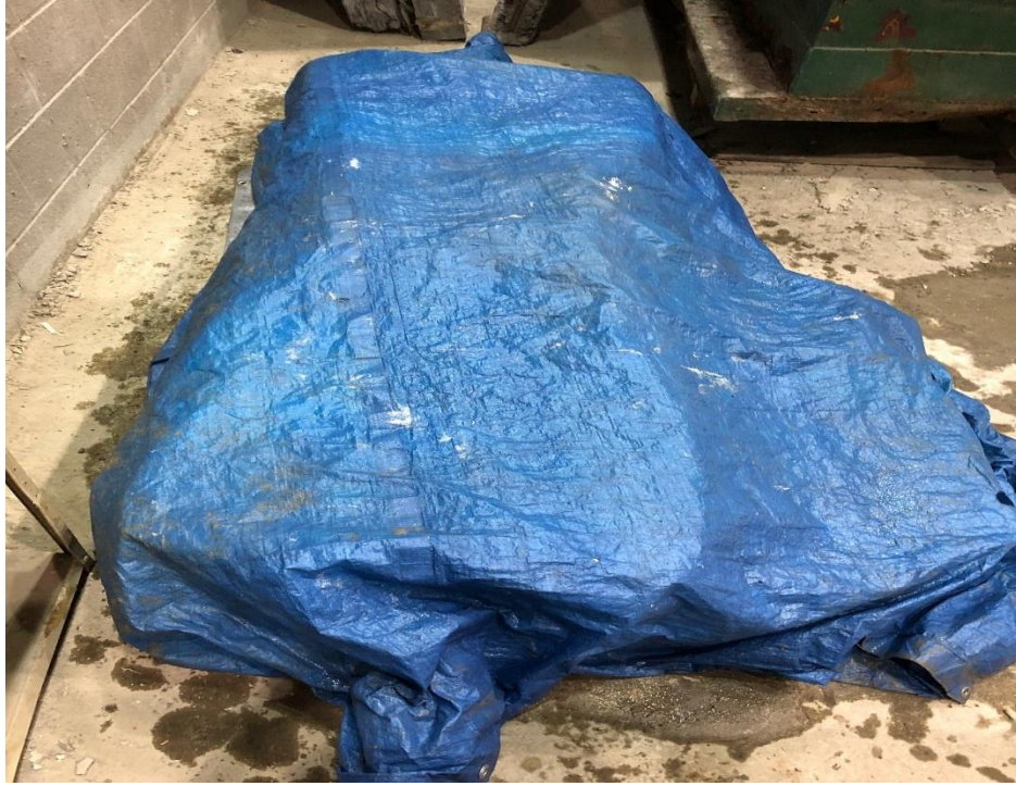
Figure 3.11: Moist curing of the RC panels after casting
