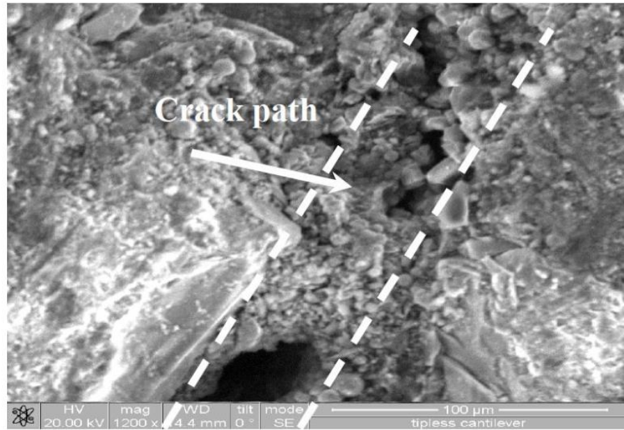
Figure2-4: ESEM micrograph of the self-healing products over the crack inside the ECC specimen after 30 days of exposure to the alkaline (sodium hydroxide) solution (Sahmaran et al., 2007; Mavani, 2012)
