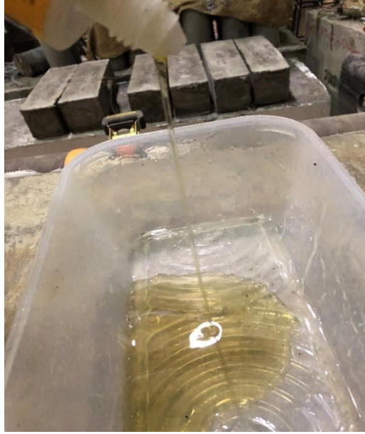
Figure 3.7: Low viscosity of the high-strength epoxy
