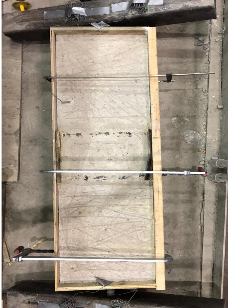
Figure 3.12: Repair layer formwork on top of the RC panel
