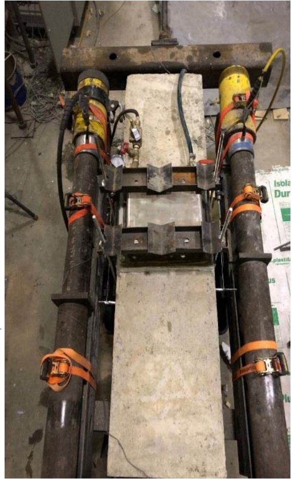
Figure 3-17: plan view of the specimen and loading test setup
