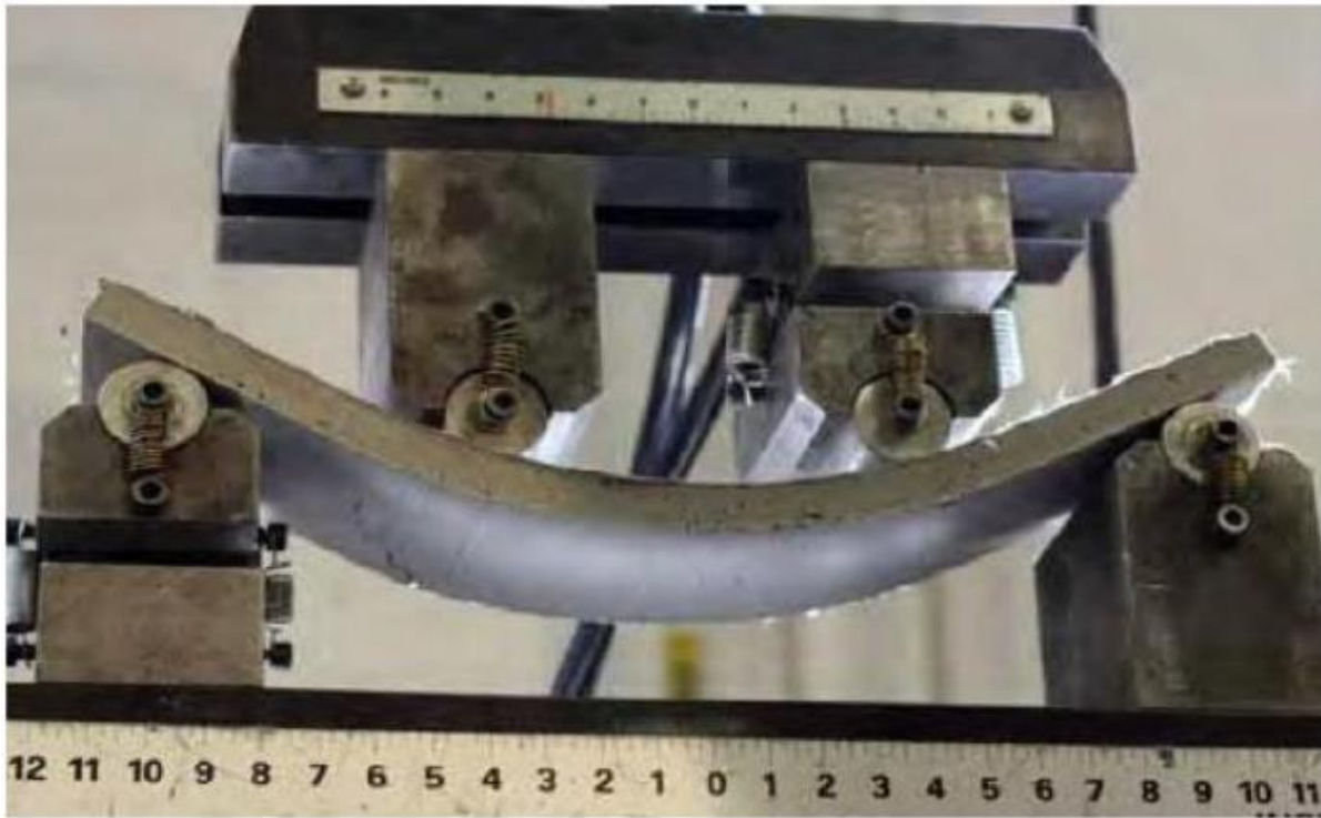
Figure 2-2: ECC beam behavior under flexural loading (Li, 2011)
