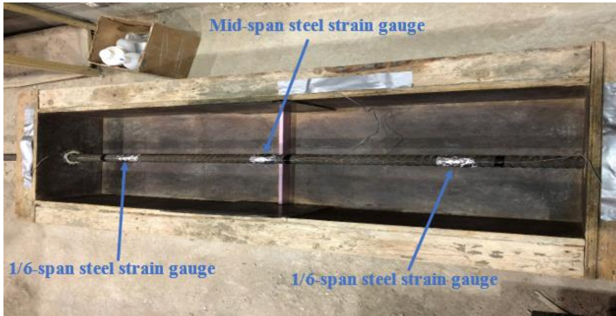
Figure 4-2: Arrangement of steel strain gauges on the rebar
