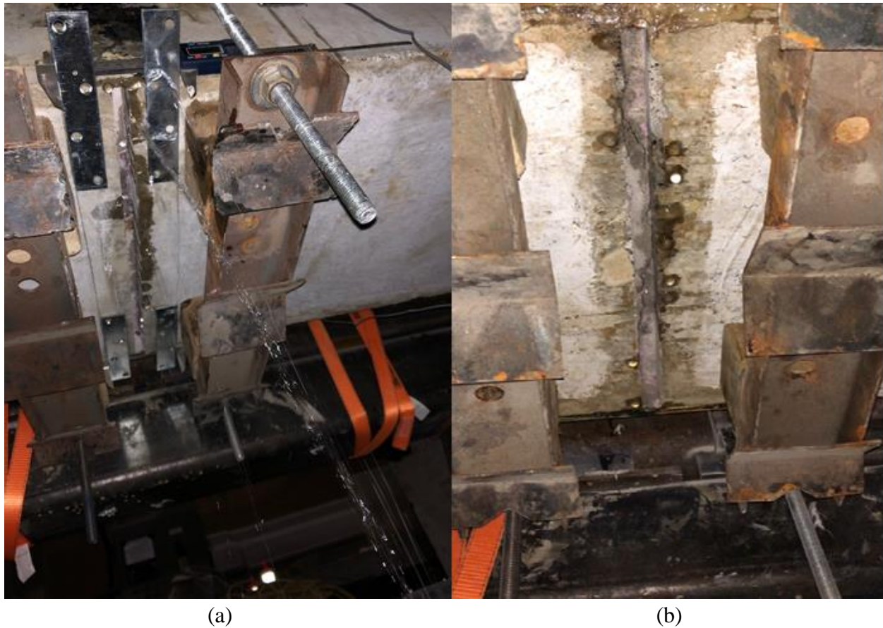
Figure 4-16: Leakage of the NC panel before and after repair using ECC slag a) Before repair b) After repair
