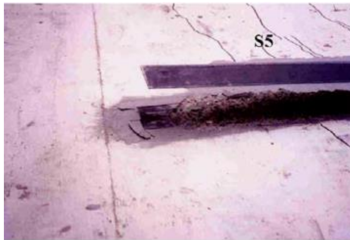
Figure 2-15: Premature failure due to CFRP strip peeling (Thanoon et al., 2005)
