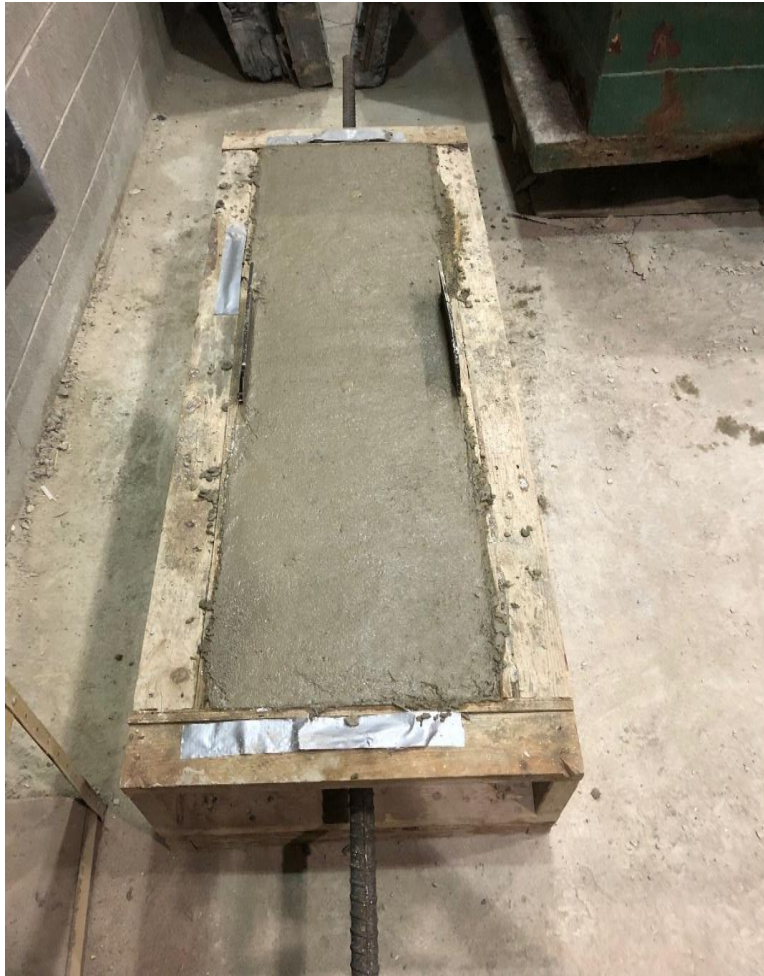
Figure 3.10: Typical reinforced normal concrete panel after casting
