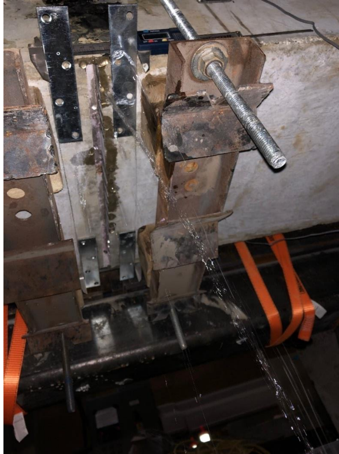
Figure 4-7: Extensive leakage in NC specimens at crack initiation (before repair)
