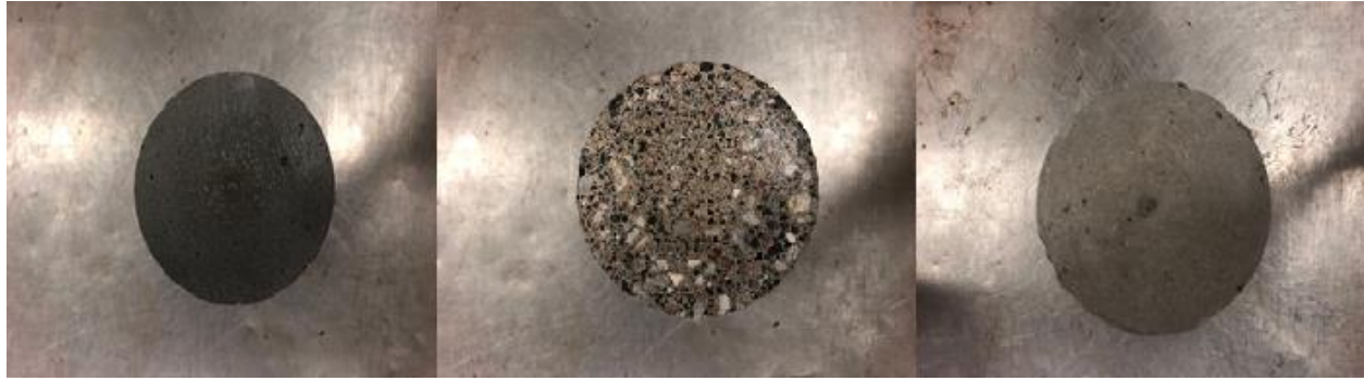
(a) ECC- Fly ash (b) NC (c) ECC- Slag Figure 3-14: Hardened cylinder specimens after grinding a) ECC- fly ash b) NC c) ECC-slag
