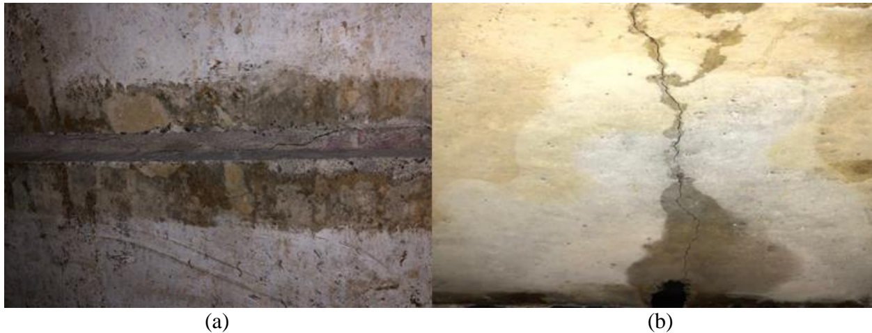
Figure 3-19: Crack formation in NC panel under direct tension a) Bottom face b) Side face
