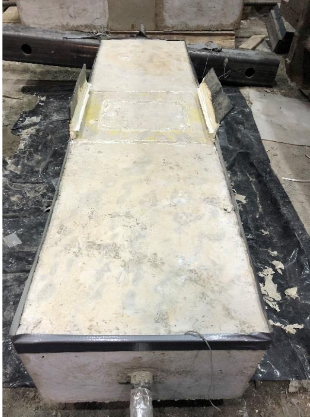
Figure 3-32: Prepared surface of the RC panel for applying GFRP
