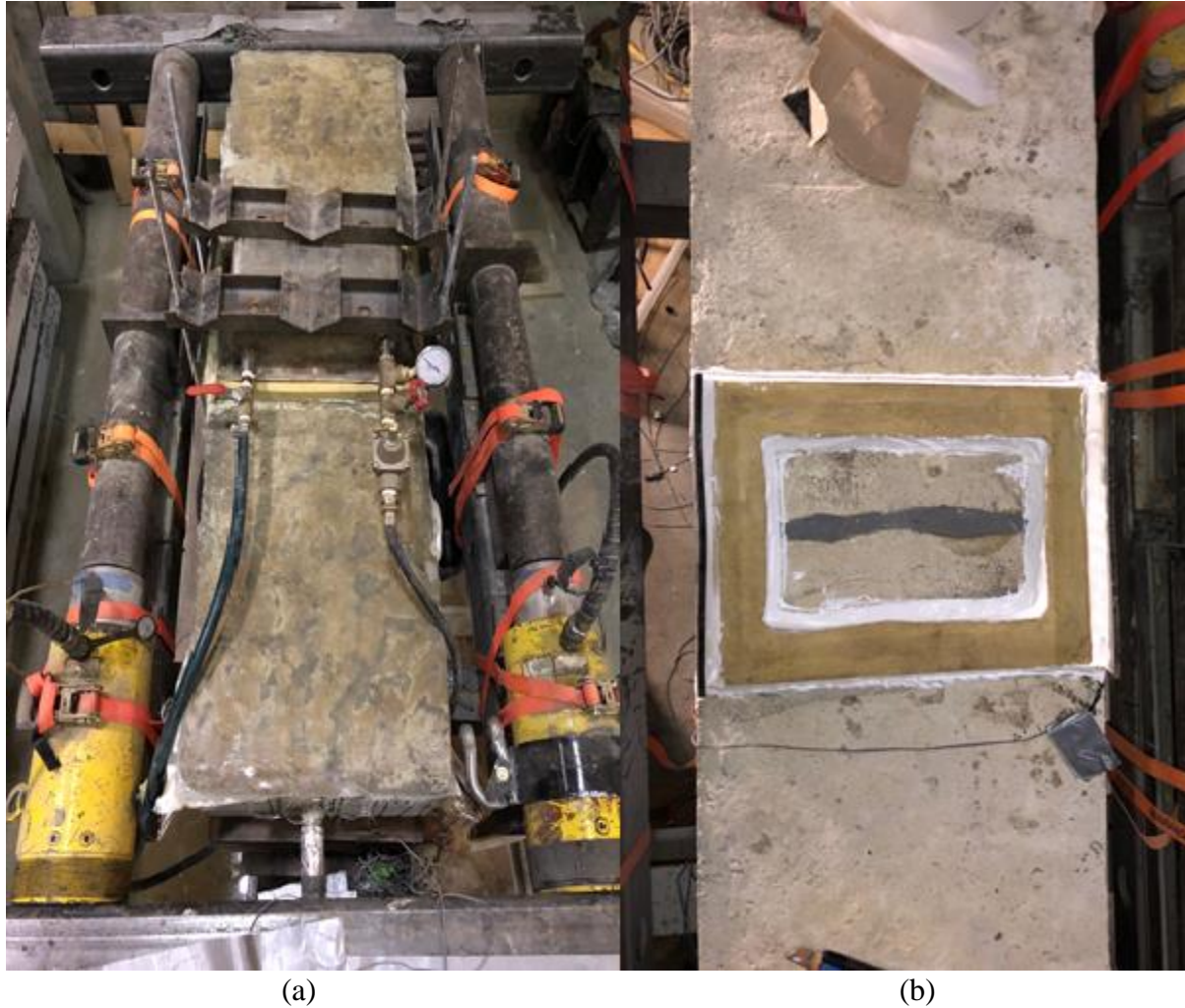
Figure 3-27: NC specimen repaired with a) GFRP laminates b) High-strength epoxy injection
