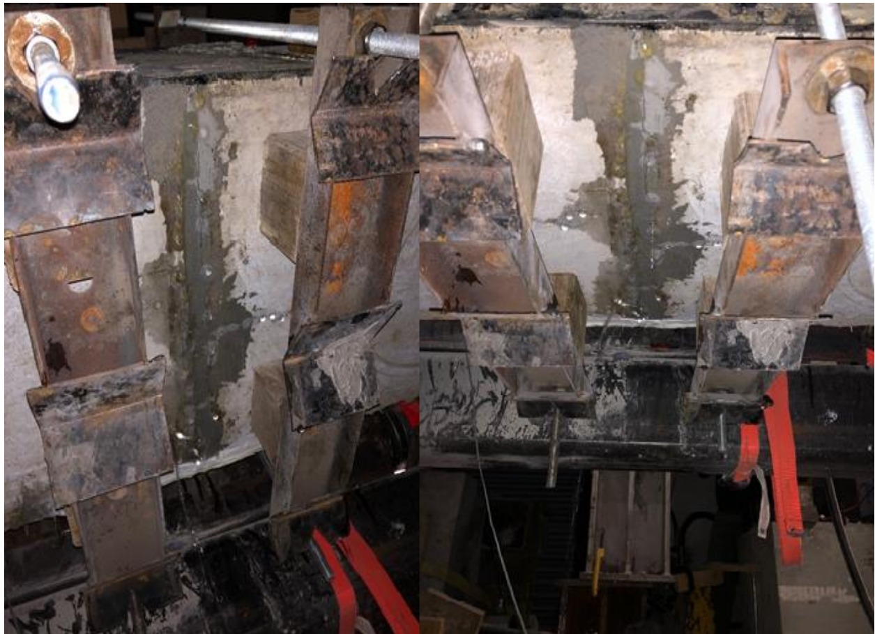
Figure 4-30: Brittle failure of the epoxy at crack location (mid-span) and high leakage rate
