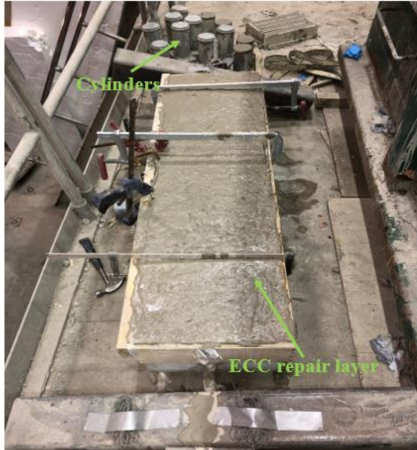
Figure 3.13: ECC repair layer after casting with control samples
