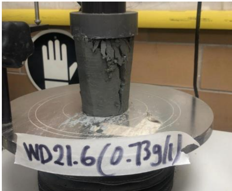
Figure 4-9: Photograph of the failure mode of a leached sample at 0.73 g/L
