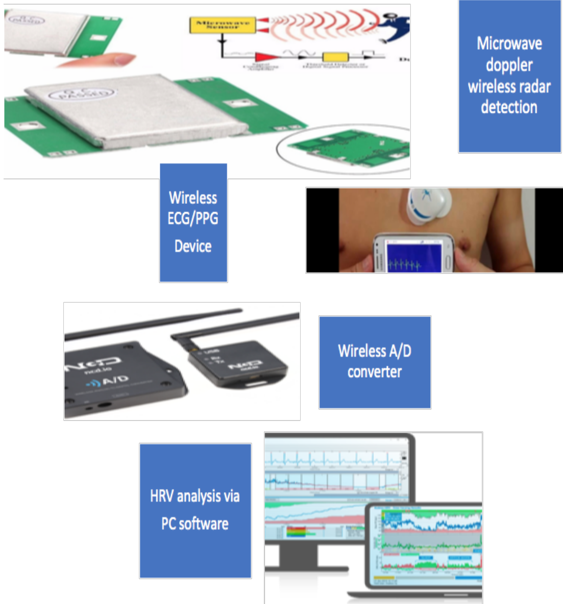
Figure 5: Telemonitoring of HRV through microwave doppler wireless radar [77], wireless ECG/PPG device [78], wireless A/D converter [79], HRV analysis software and internet.
