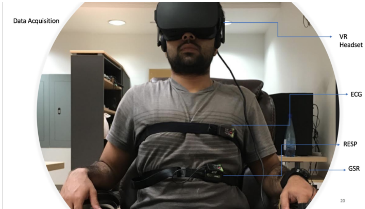
Figure 14: Data acquisition through wireless ECG, GSR and RESP devices
