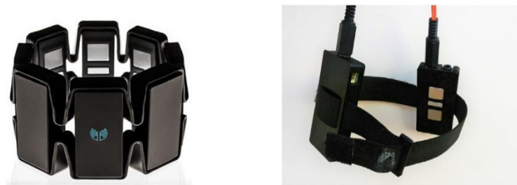
Figure 4. This figure shows the Myo band on the left and two EMG channel sensors on the right. Image source: [21,22].
