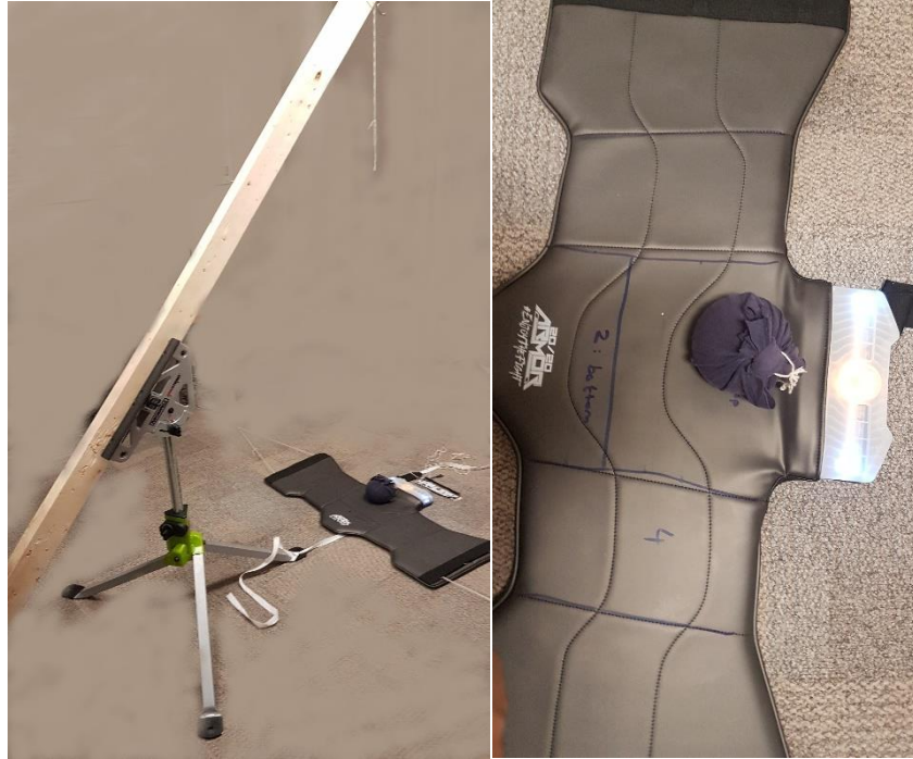
Figure 14. This figure shows the SARput - drop-test apparatus (left) and the drop location (right). The vest is tied into place using anchor points.
