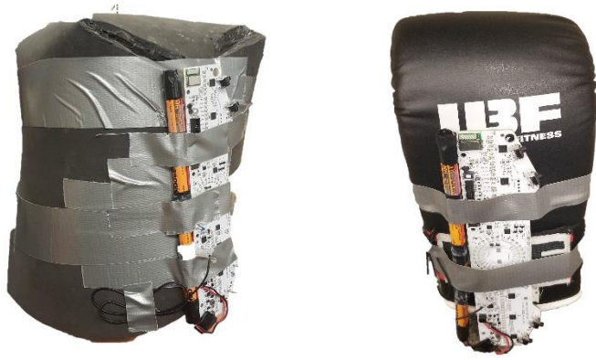
Figure 24. This figure shows the eHelmet with 20/20 board and IBF glove with 20/20 Board
