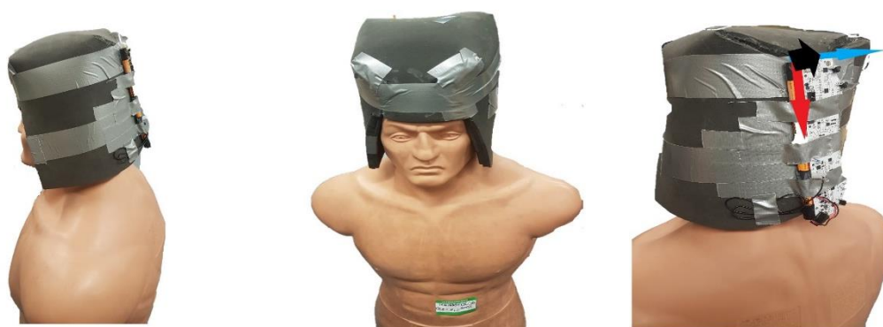
Figure 32. This figure shows the eHelmet made of the smart foam material as well as the x-y-z axis relative to the board. Note, red: y-axis, blue: x-axis, black: z-axis (out of page)
