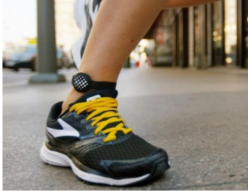
Figure 6. This figure shows the Moov Now device that contains nine-axis motion sensing. Image source: [29].
