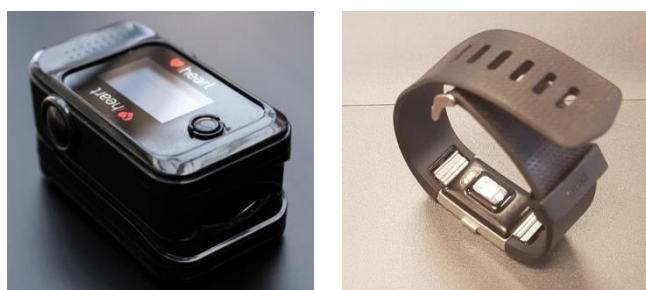
Figure 3. This figure shows the finger-tip (iHeart) sensor on the left and the wrist (Fitbit Charge 2) sensor on the right Image source: [18].
