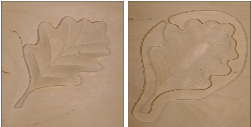
Image 40-41: Hand-carved leaf (left) | Digitally-fabricated leaf (right)
