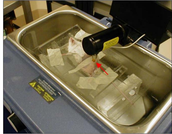
Fig. 1. Setup to immobilize the mammary tissue of the mouse in the heated water bath which was used as a coupling medium. The transducer (indicated by the arrow) was scanned linearly across the mammary tissue.
