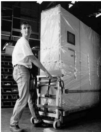
Fig. 2. A transport device to eliminate manual lifting and carrying .
