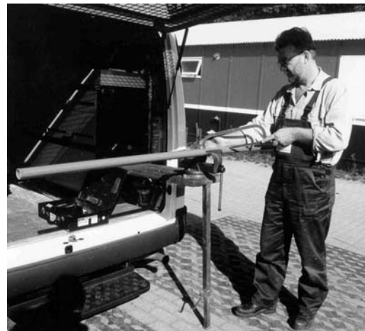
Fig. 1. Draw-out work-bench to prevent working on the floor and reduce back flexion
