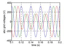
Fig. 7. Grid Voltages. 50% dip type C.
