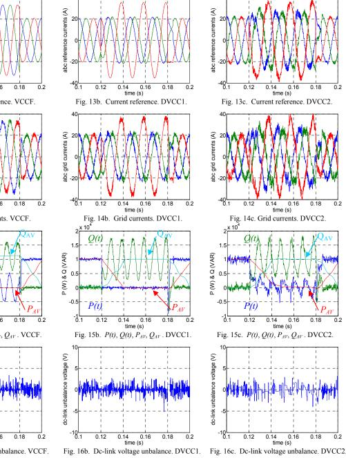
When a grid dip appears, the current reference is changed to meet LVRT requirements. Current reference tracking performance given by the predictive controller is fast, accurate and presents no overshoot. All the three considered controllers comply with the LVRT requirements.
