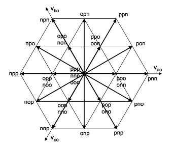
Fig. 6. Possible voltage vectors and switching states generated by a three-level inverter.
