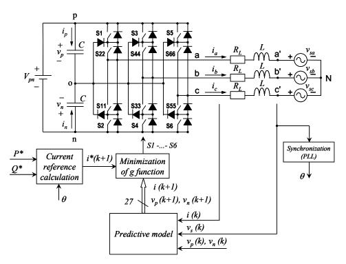
Fig. 4. NPC converter connected to the grid through a L filter and simplified control block diagram.
