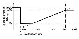
Fig. 1. Voltage limit curve to allow wind turbine disconnection.
