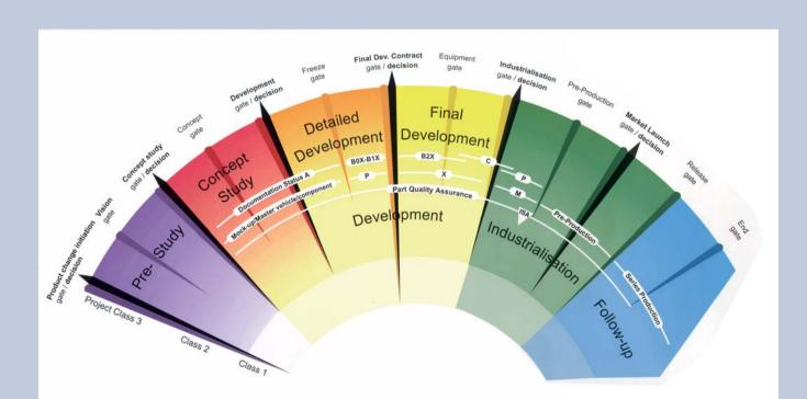
**Fig. 2.** The Volvo Corporation has developed a 'Global Development Process' GDP, which describes development processes with regard to new products and production systems. The built-in check-points, 'gates', cannot be passed until all demands at the previous level have been met. Volvo Powertrain in Skövde, in the light of the described research project, has begun to integrate ergonomics and working environment in the GDP.
