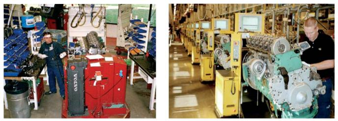
For several years, the National Institute for Working Life has monitored work at Volvo Powertrain in Skövde. During 2002, a reorganization was carried out with which the earlier model with 'docks' for parallel production (left picture) with an assembly worker in each one, was replaced by a serial production system with an assembly line (right picture).
