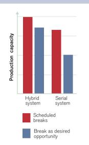
**Fig. 5.** Ergonomics in simulated flows. A comparison of production systems when a 'break as desired opportunity' is introduced.
