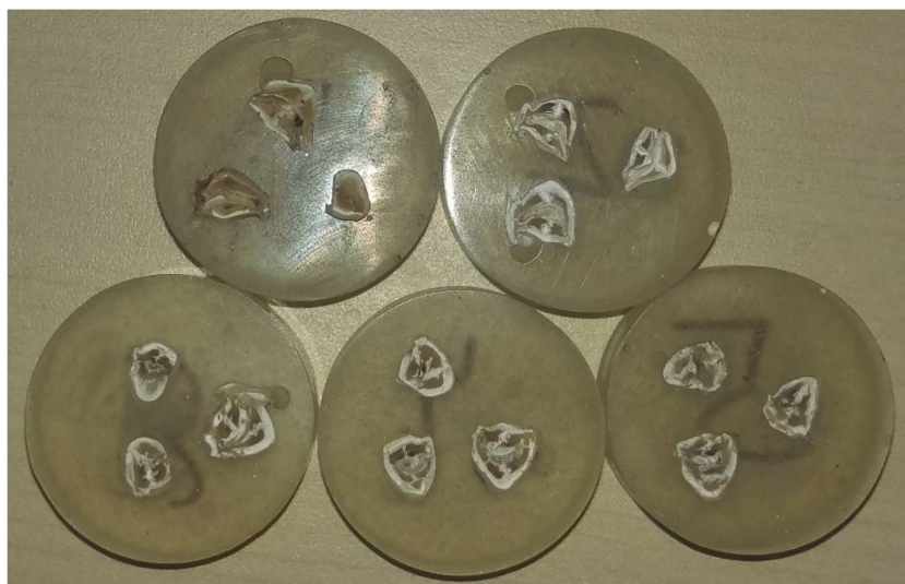
Figure 8. Dental pucks mounted in resin and with their buccal surfaces exposed. Picture was taken after they were brushed.
