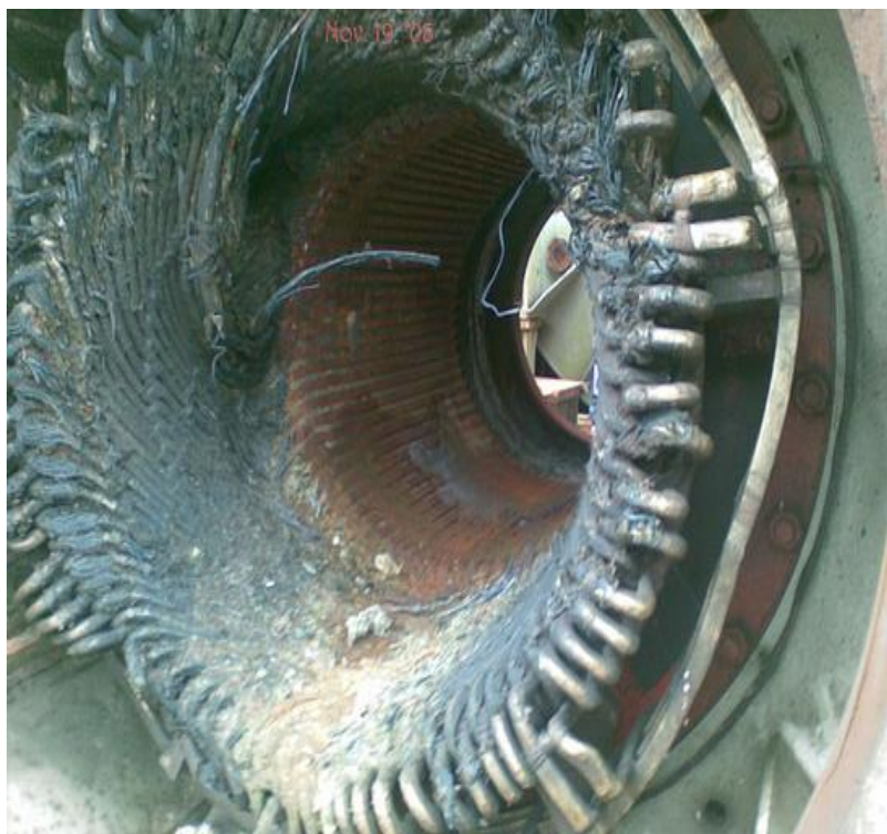
Figure 34: Turbine generator after fault
