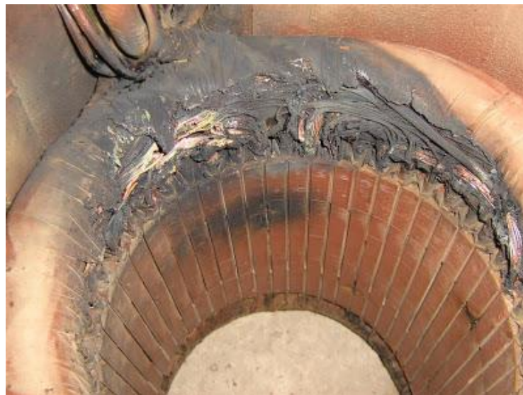
Figure 80: Motor Winding failure
