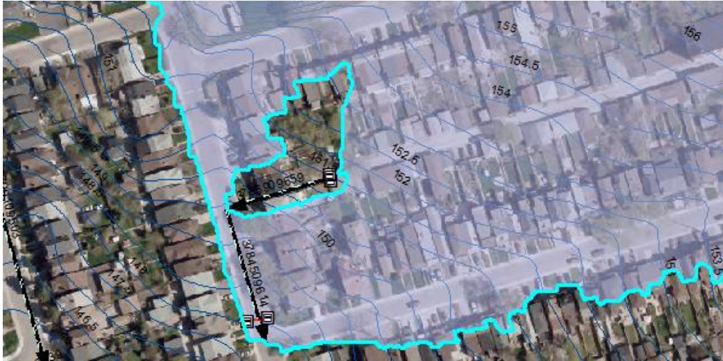
Figure 62. Error # 3 Subcatchment containing another smaller subcatchment
