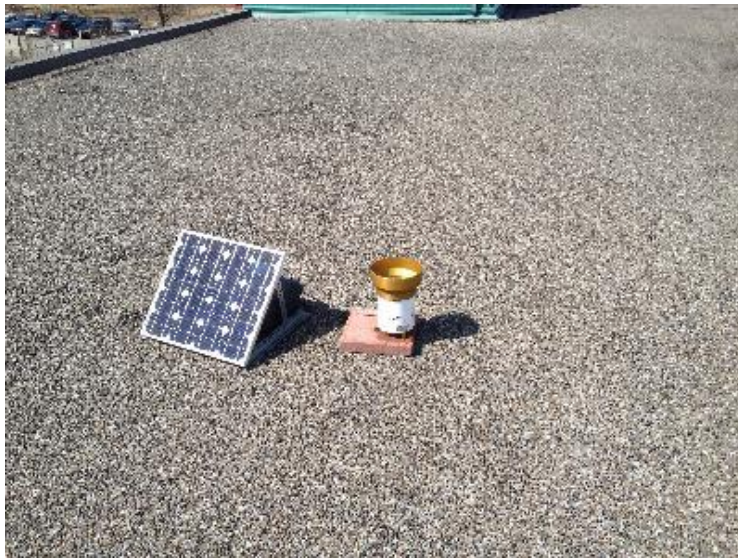
Figure 33. RG-020 which is a tipping bucket style rain gauge known as the TR-525USW rain gauge (Cole, 2014a)
