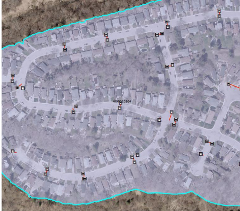
Figure 61. Error # 2 Subcatchment contains multiple sets of catch basins belonging to multiple pipes
