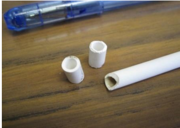
Figure 6.16 Photo of the ceramic broken pieces used to fit into the SEM imaging analyzer.
