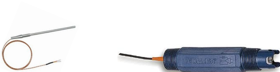
Figure 6.10 Temperature (left) and pH (right) sensors that are connected to the data acquisition system
