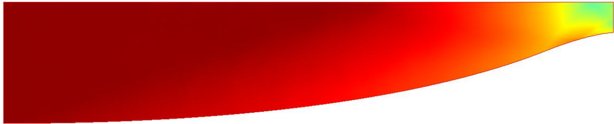
Figure 9.16 shows final filled Mach number contours (800000 time steps).
