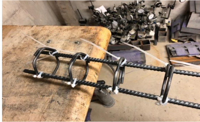
Figure 18. Binding tie bars and longitudinal bars using zip ties
