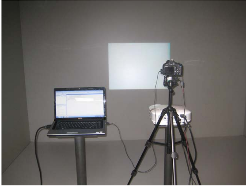
Figure 5.1: The full setup of the system which includes: LCD projector, camera, and laptop.
