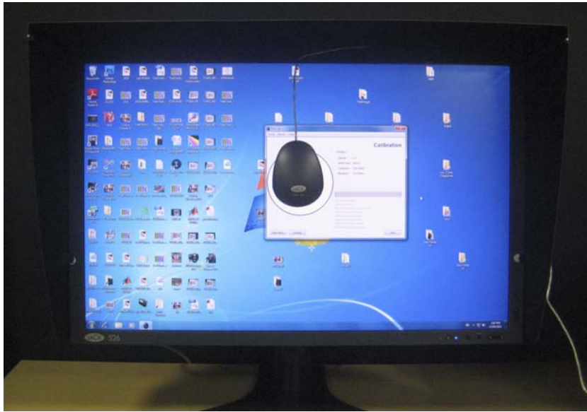
Figure 2.5: LaCie 526 monitor with blue eye measuring instrument during calibration process.
