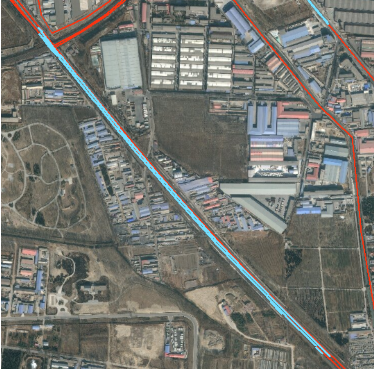
Fig 5.5: Visual Inspection of Extracted Road Network (Highlighted Blue Line) Overlaid with Aerial Photograph Provide by ESRI, and Road Centerline from www.openstreetmap.org (Red Lines) in Region 1.
