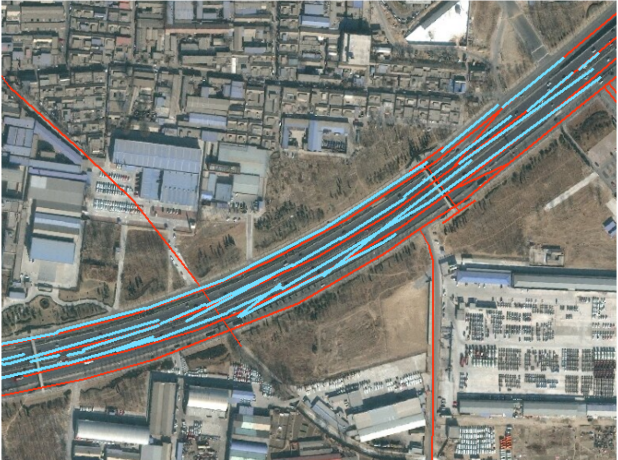
Fig 5.6: Visual Inspection of Extracted Road Network (Highlighted Blue Line) Overlaid with Aerial Photograph Provide by ESRI, and Road Centerline from www.openstreetmap.org (Red Lines) in Region 2.
