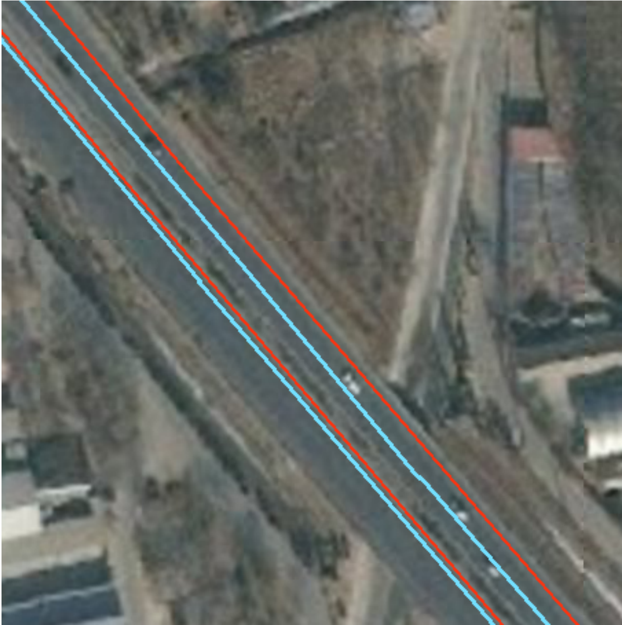
Fig 5.8: Close-Up Views of Extracted Road Network (Highlighted Blue Line) Overlaid with Aerial Photograph Provide by Esri, and Road Centerline from www.openstreetmap.org (Red Lines) in Region 1.
