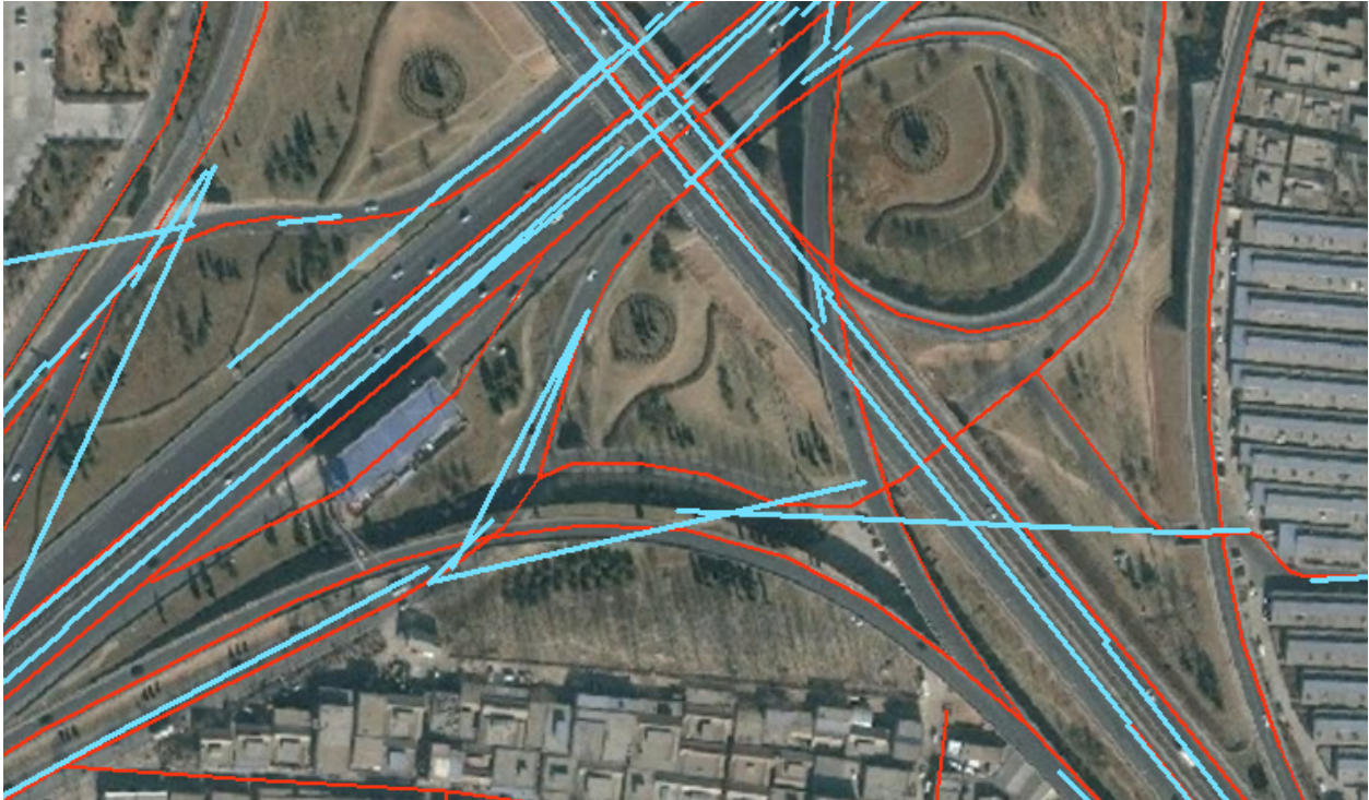
Fig 5.10: Close-Up Views of Extracted Road Network (Highlighted Blue Line) Overlaid with Aerial Photograph Provide by ESRI, and Road Centerline from www.openstreetmap.org (Red Lines) in Region 2.
