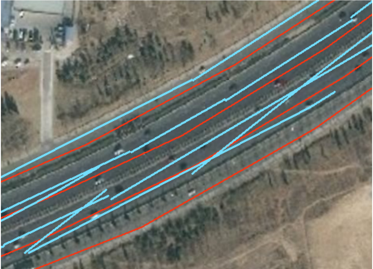
Fig 5.9: Close-Up Views of Extracted Road Network (Highlighted Blue Line) Overlaid with Aerial Photograph Provide by ESRI, and Road Centerline from www.openstreetmap.org (Red Lines) in Region 2.
