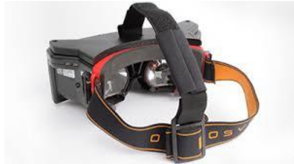
(b) Head mounted video-based eye gaze tracker, suitable to graphical interactive systems.
