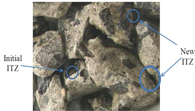
Figure 2.2 Interfacial Transition Zones (ITZs) locations on RCA concrete (Ryu, 2002)
