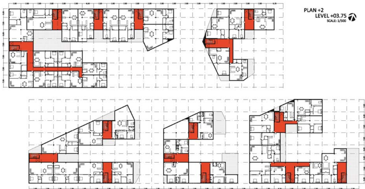
Figure 67: A typical plan of building apartments with multiple-staircase/elevator concept. Source: Author
