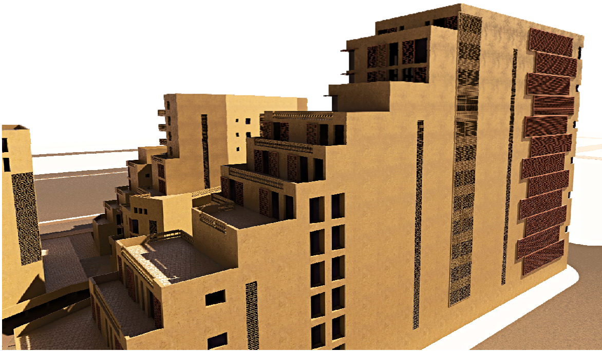
Figure 89: View to the north-west facade with horizontal fabric shading. Source: Author
