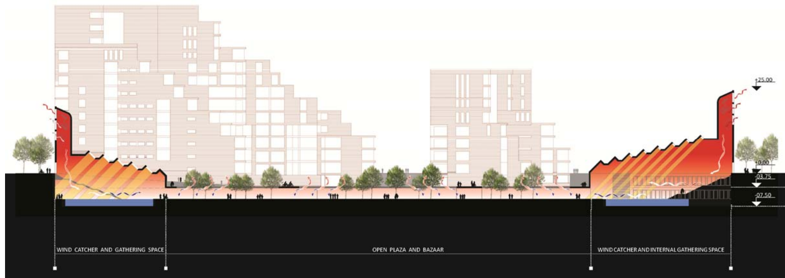
Figure 69: Behaviour of wind inside the block. Source: Author
