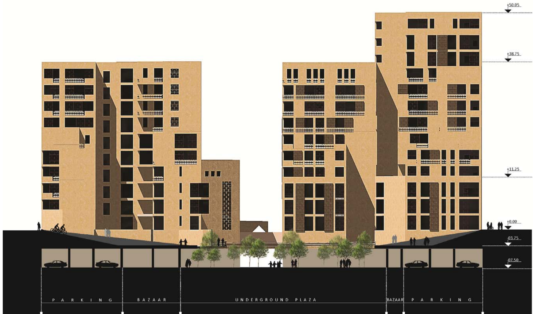
Figure 66: North-South site Section through the neighbourhood, showing the mixed-used characteristic of the proposed city block. Source: Author
