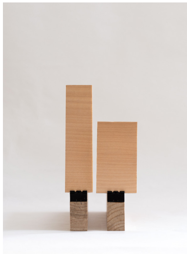
Figure 7-13 Impact of aspect ratio on response
