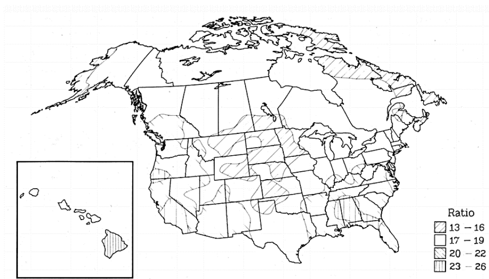
Figure 4.2.1 – Leakage infiltration ratio ( N_o ) (Sherman, 1987)
