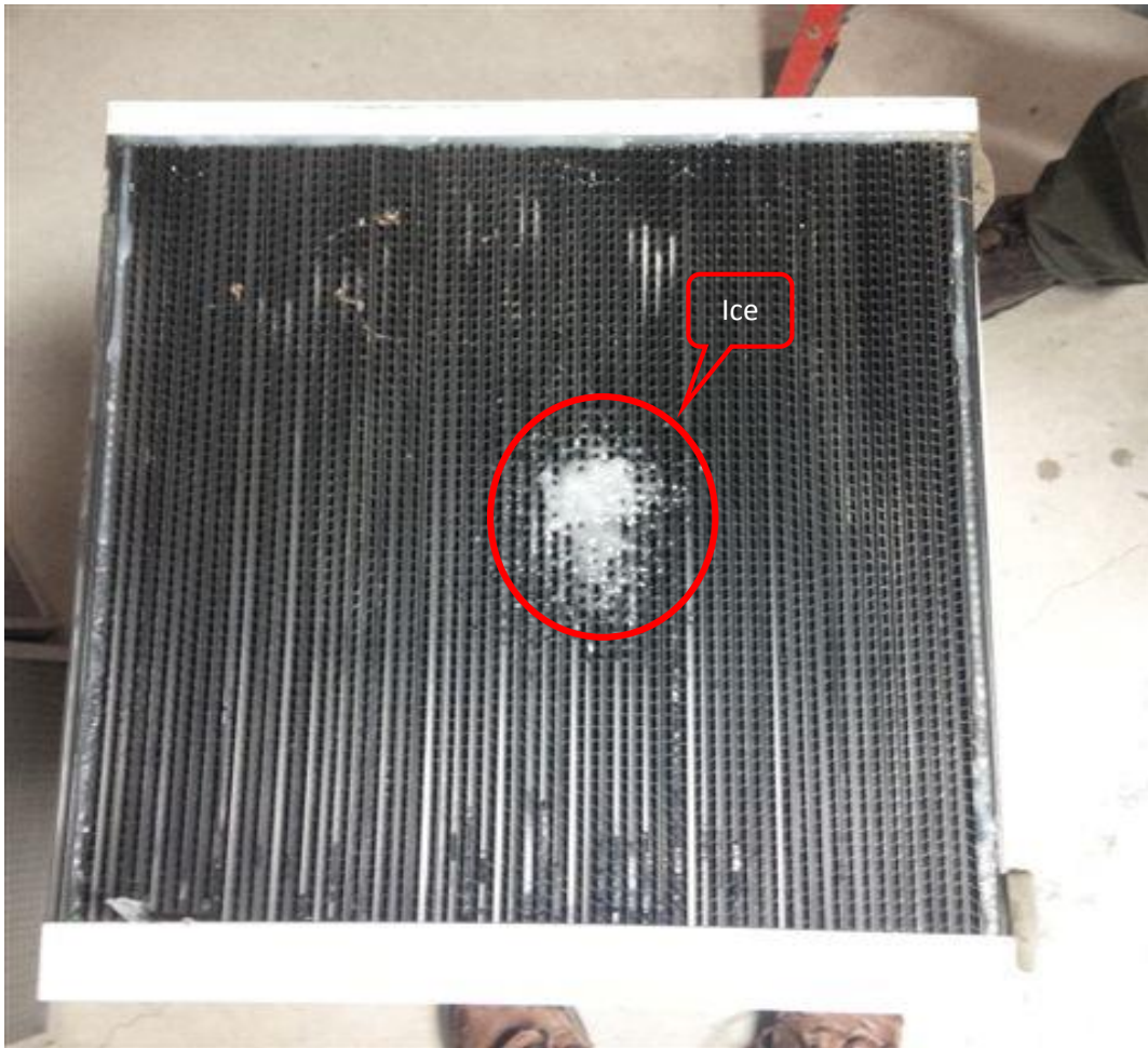
Figure 6.6.1 – Ice formation inside the sensible core of the HRV
