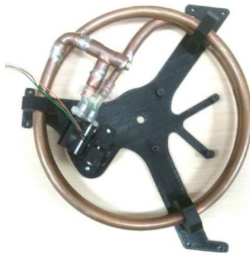
Figure 1.5: Pumped Fluid Loop Actuator Assembly [27]
