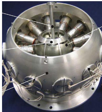
Figure 1.4: Spherical Electromechanical Actuator Assembly [9]
