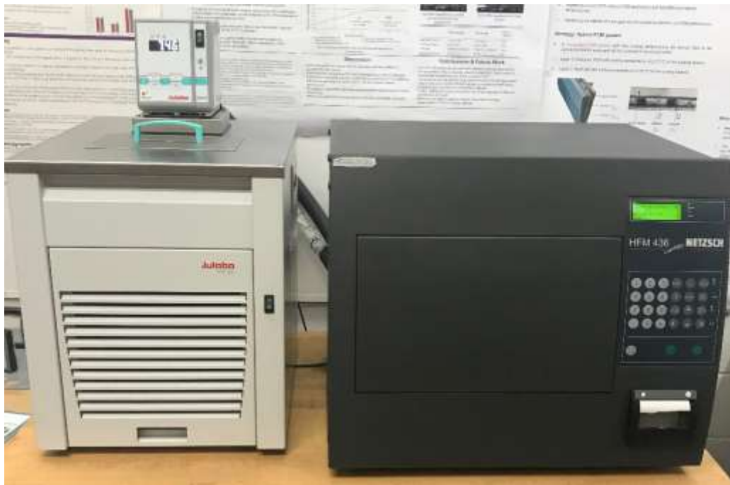
Figure 3.2: Heat flow meter NETZSCH HFM 436 Lambda apparatus
