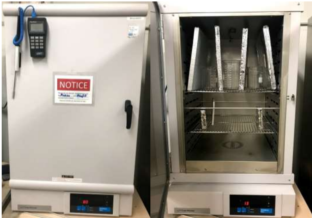
Figure 3.5: Mechanical convection oven used for elevated temperature ageing
