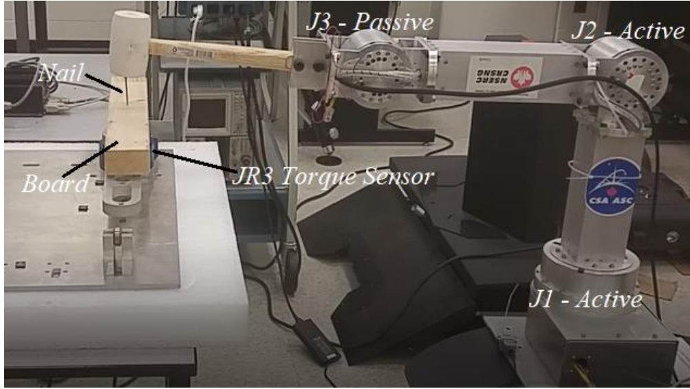
FIGURE 20 DIAGRAM OF MRR WITH HAMMER END-EFFECTOR
