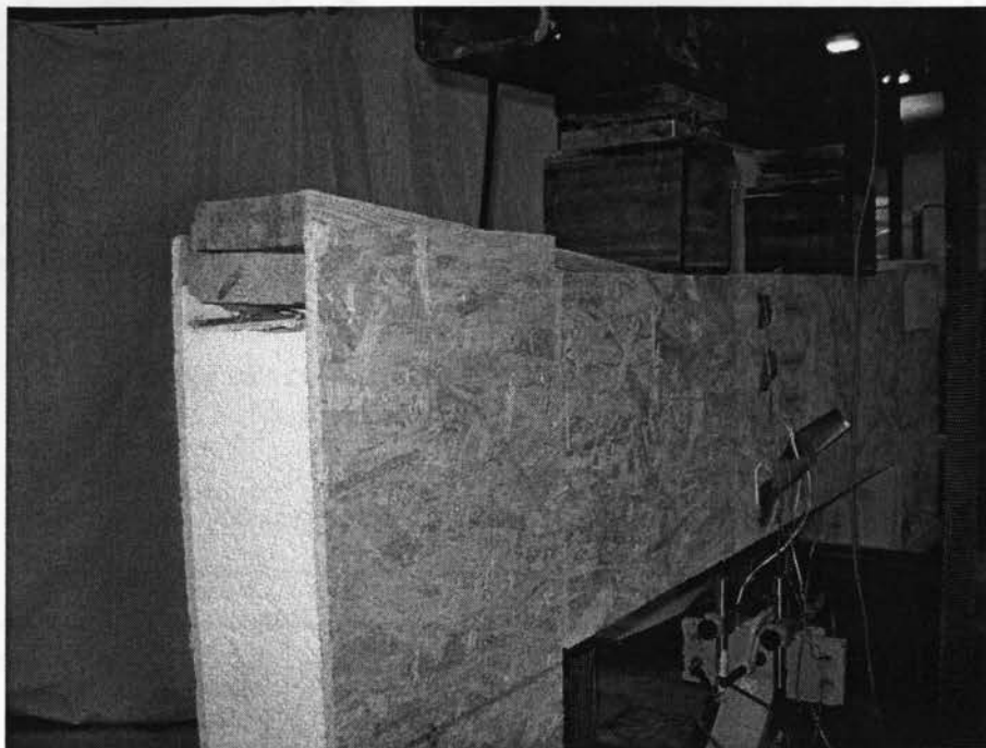
Figure 4.2 Close-up view of the failure mode in the left side of header H-1
