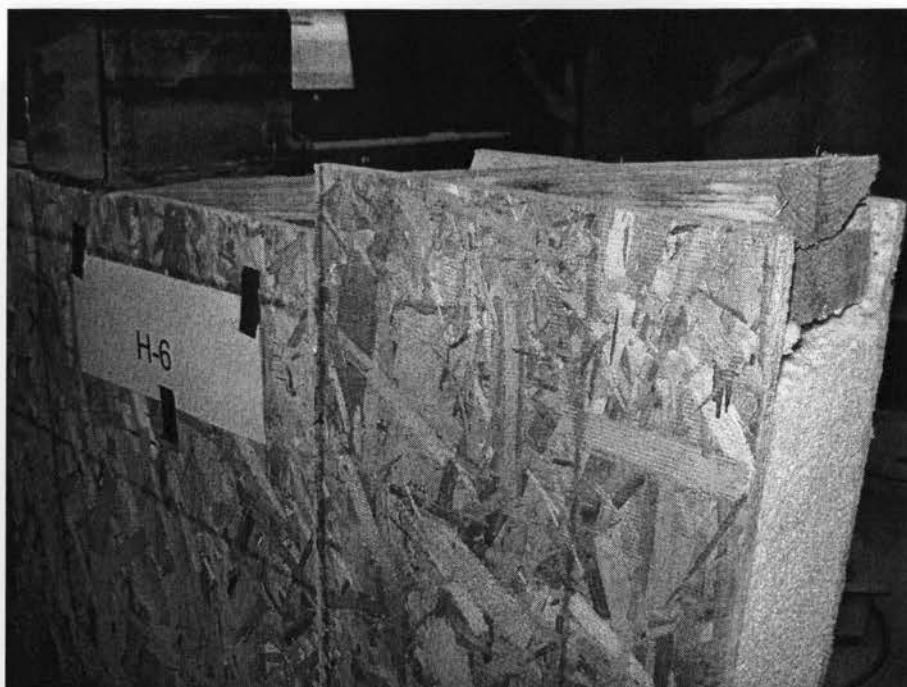
Figure 4.27 Close-up view of the failure mode of the right side of header H-6
