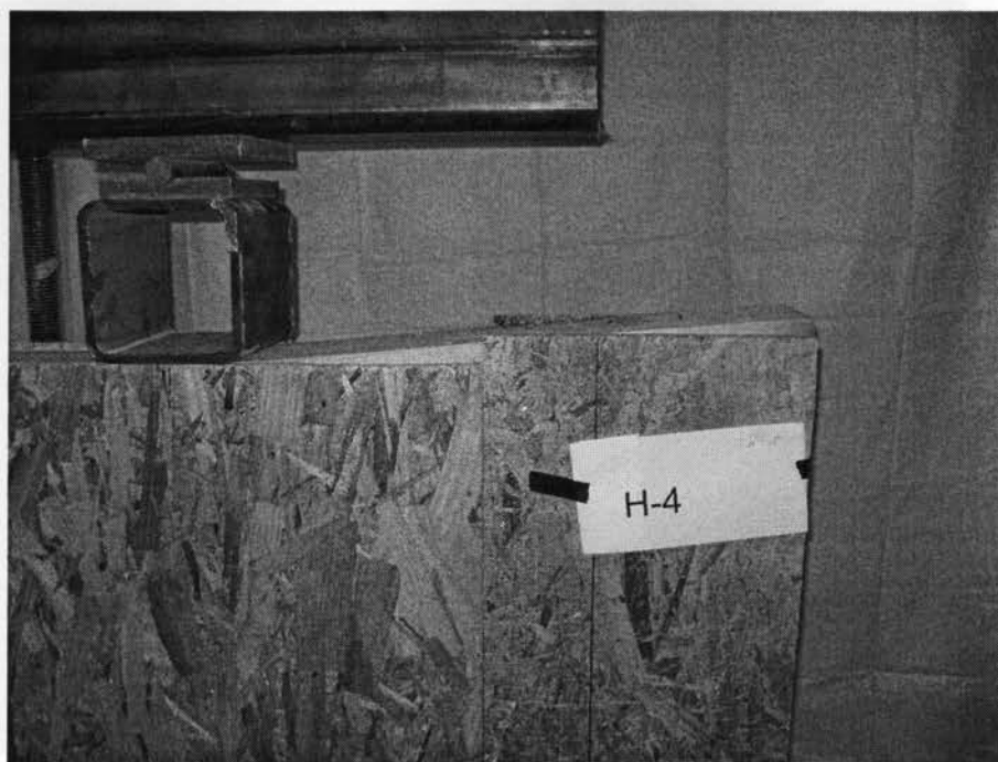
Figure 4.17 Close-up view of the failure mode of the right side of header H-4
