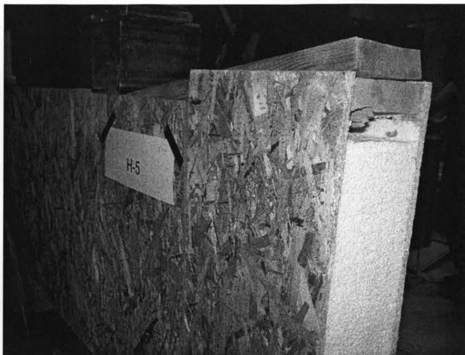
Figure 4.22 Close-up view of the failure mode of the right side of header H-5
