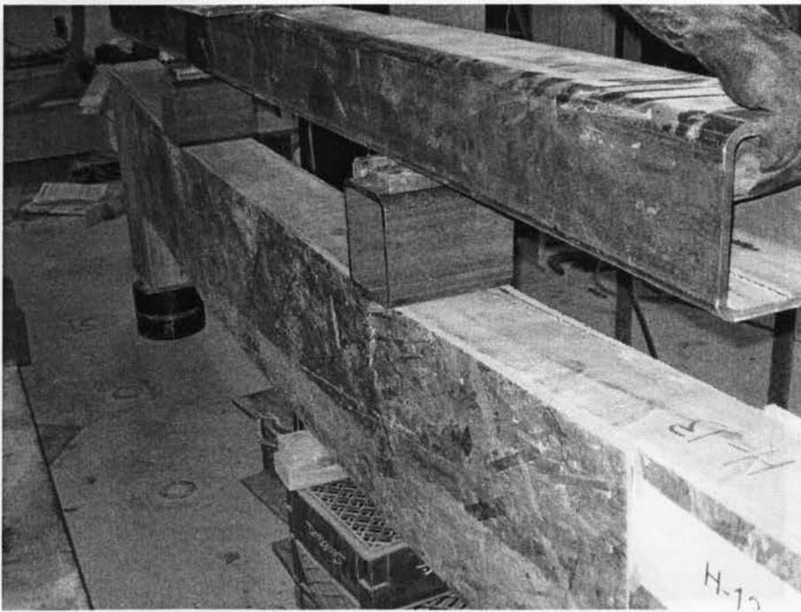
Figure 4.61 View of header H-13 after failure
