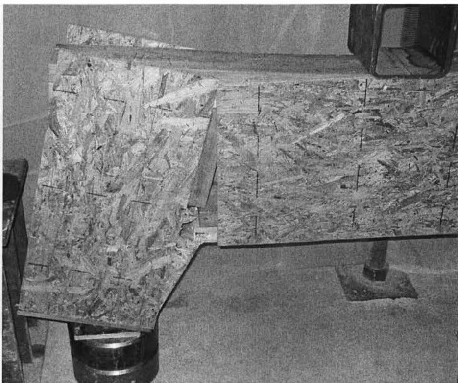
Figure 4.46 Close up view of the failure mode of header H-9
