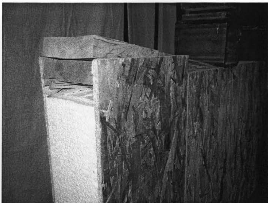
Figure 4.23 Close-up view of the failure mode of the left side of header H-5
