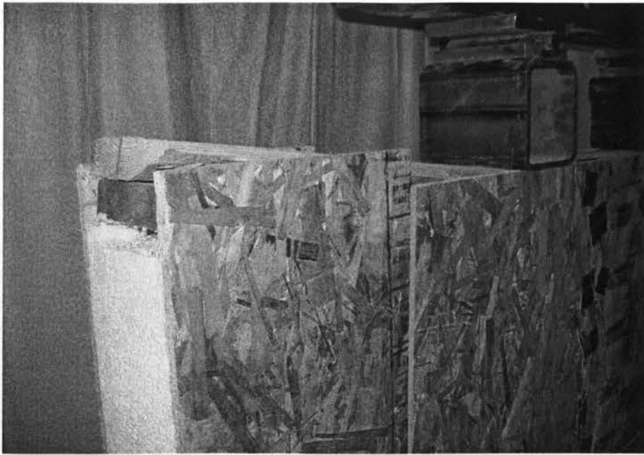
Figure 4.28 Close-up view of the failure mode of the left side of header H-6
