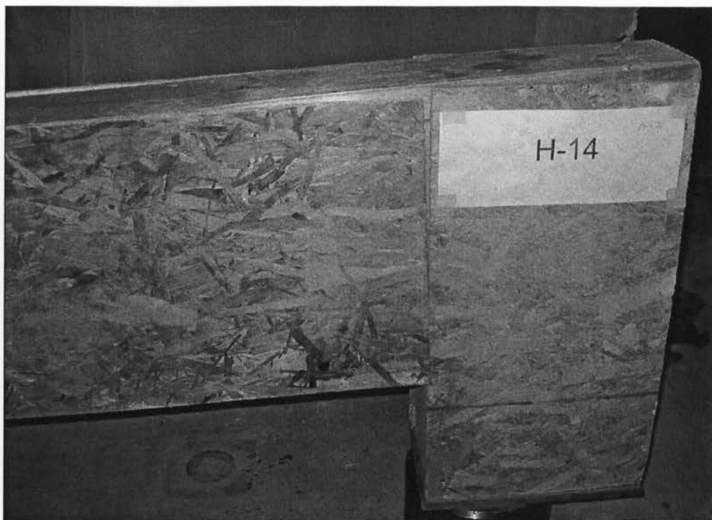
Figure 4.71 Close-up view of the failure mode at support of header H-14
