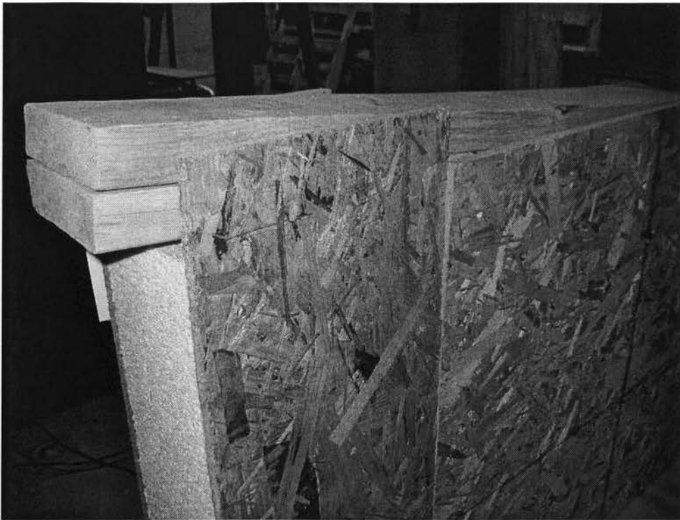
Figure 4.90 Close-up view of the failure mode at left support of header H-17
