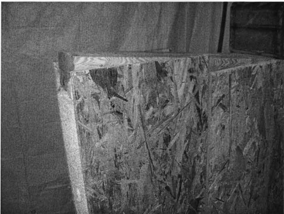
Figure 4.19 Close-up view of the failure mode of the left side of header H-4
