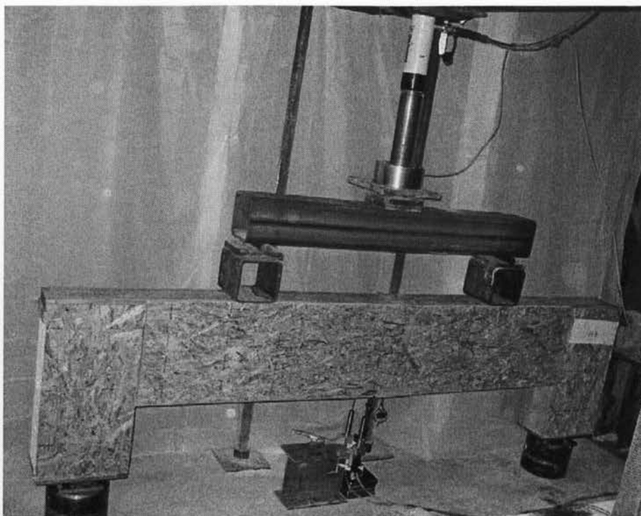
Figure 3.20 View of setup on steel rollers for header H-9 before testing
