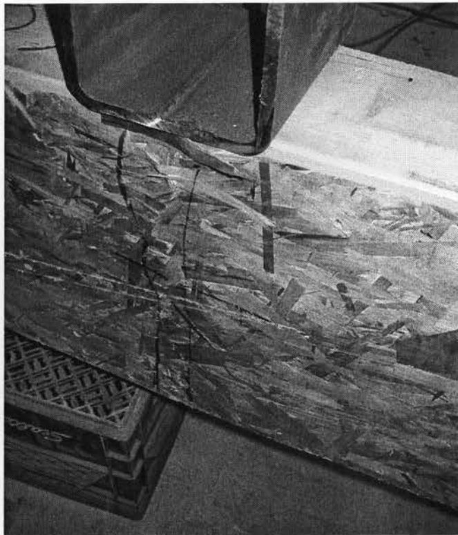
Figure 4.65 Close-up view of the flexure failure mode at quarter point of header H-13
