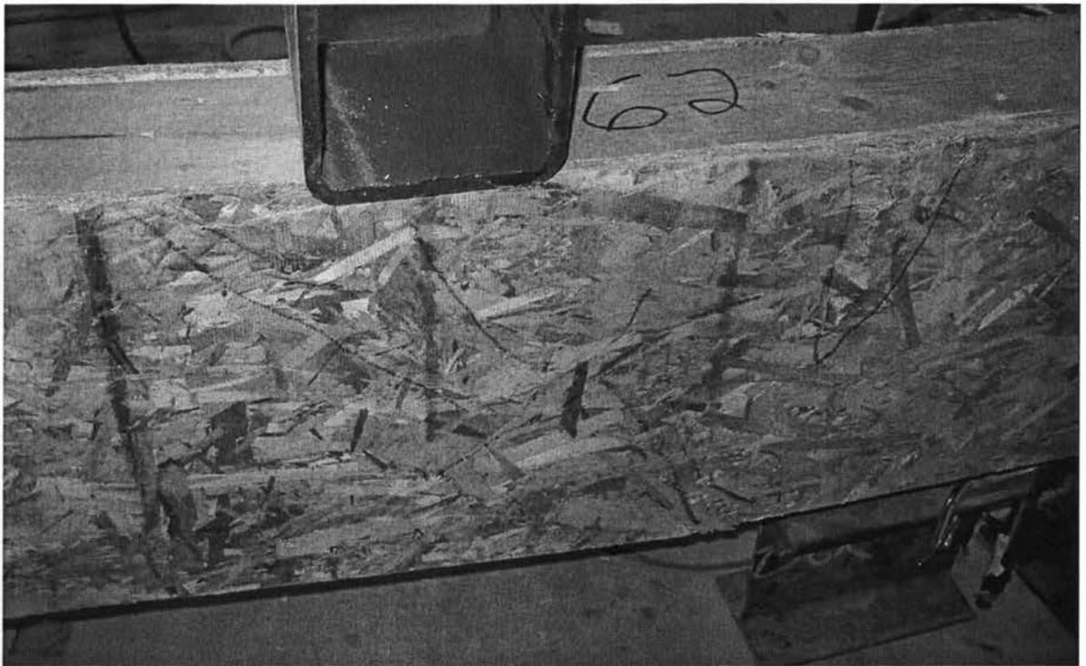
Figure 4.73 Close-up view of the flexure failure mode between quarter point and mid-span of header H-14
