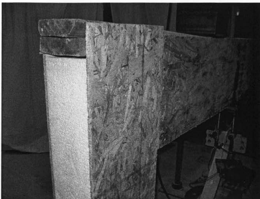
Figure 4.40 Close-up view of the failure mode of the left side of header H-8
