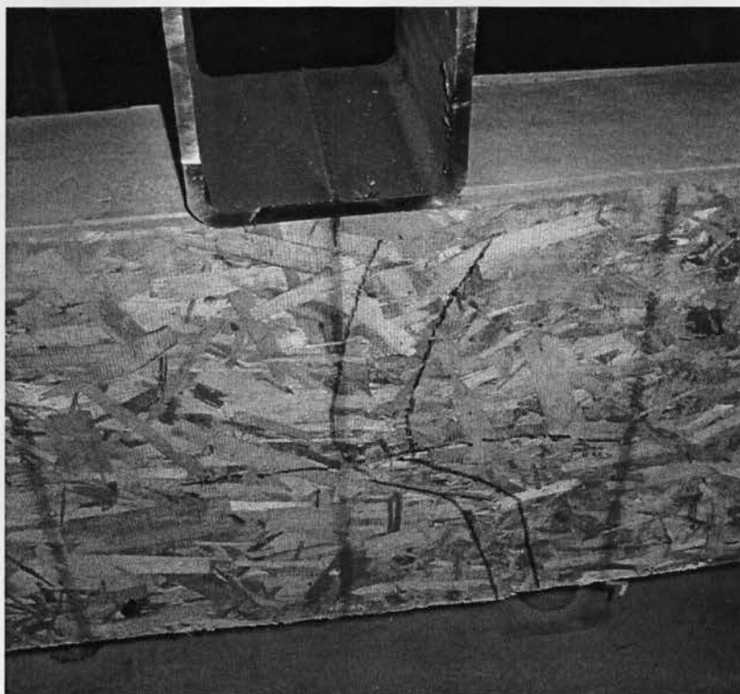
Figure 4.68 Close-up view of the flexure failure mode at quarter point of header H-13
