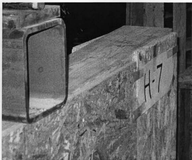
Figure 4.33 Close-up view of the failure mode of the right side of header H-7
