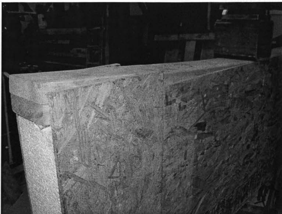
Figure 4.85 Close-up views of the failure mode at supports of header H-16
