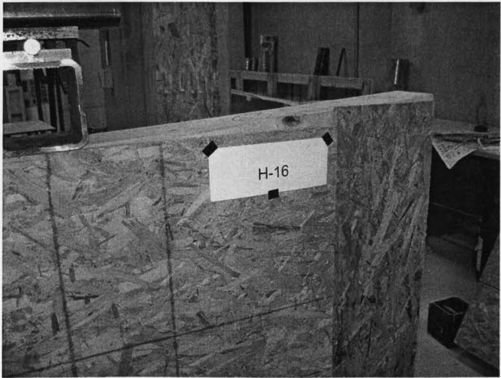
Figure 4.84 View of header H-16 after failure
