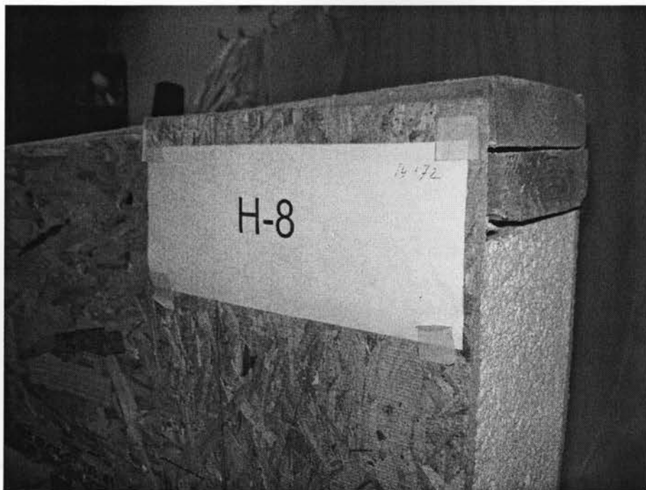
Figure 4.39 Close-up view of the failure mode of the right side of header H-8
