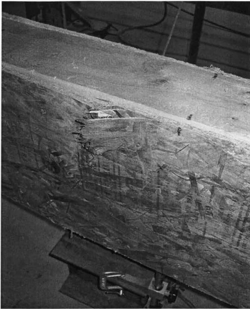
Figure 4.79 Close-up view of flexure failure mode at front side of mid-span of header H-15
