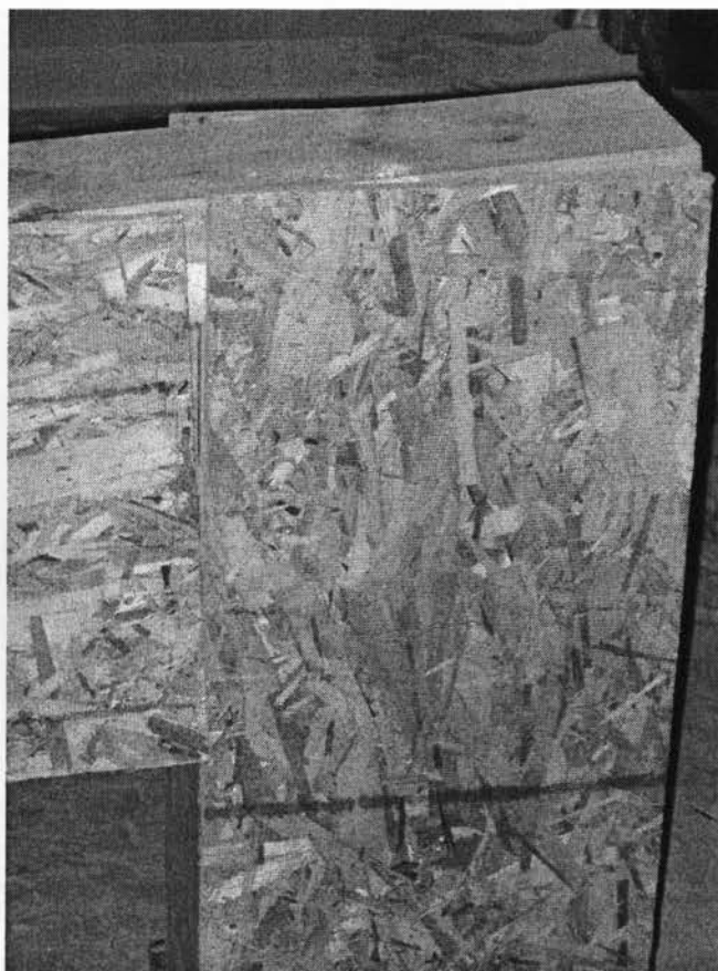
Figure 4.82 Close-up view of the failure mode at support of header H-15
