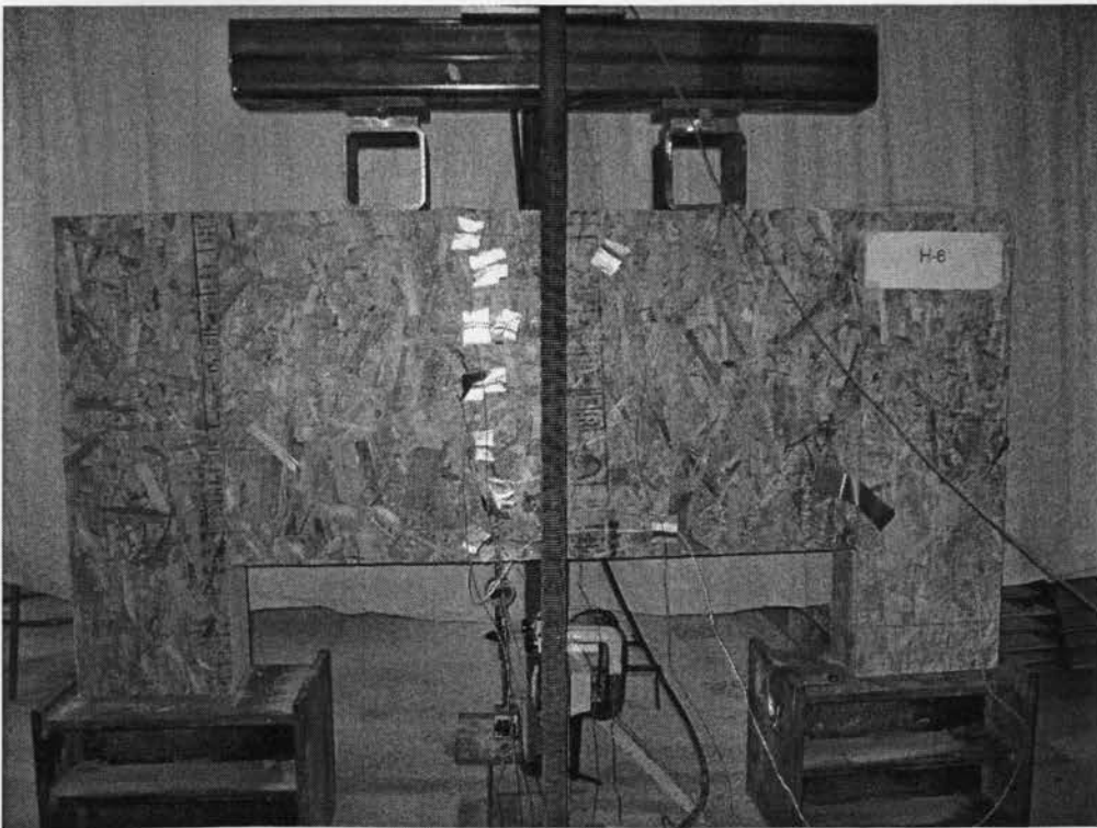
Figure 3.17 View of setup for header H-6 before testing
