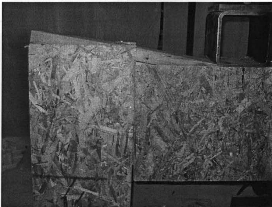
Figure 4.12 Close-up view of the failure mode of header H-3
