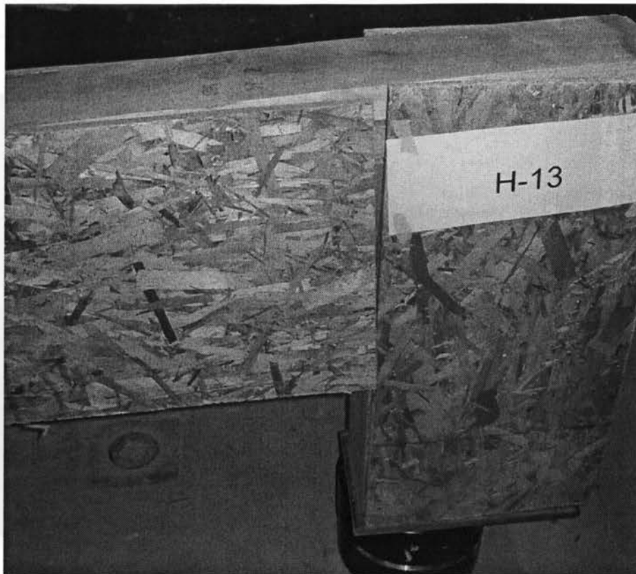
Figure 4.62 Close-up view of the failure mode at support of header H-13
