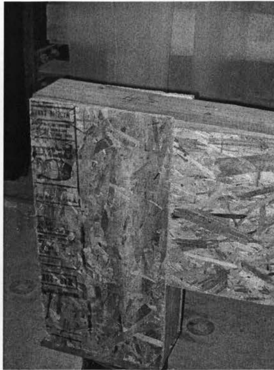
Figure 4.34 Close-up view of the failure mode of left side of header H-7
