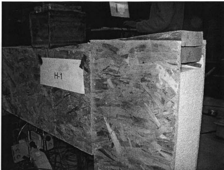
Figure 4.3 Close-up view of the failure mode of the right side of header H-1
