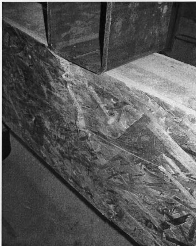
Figure 4.66 Close-up view of the flexure failure mode at quarter point of header H-13
