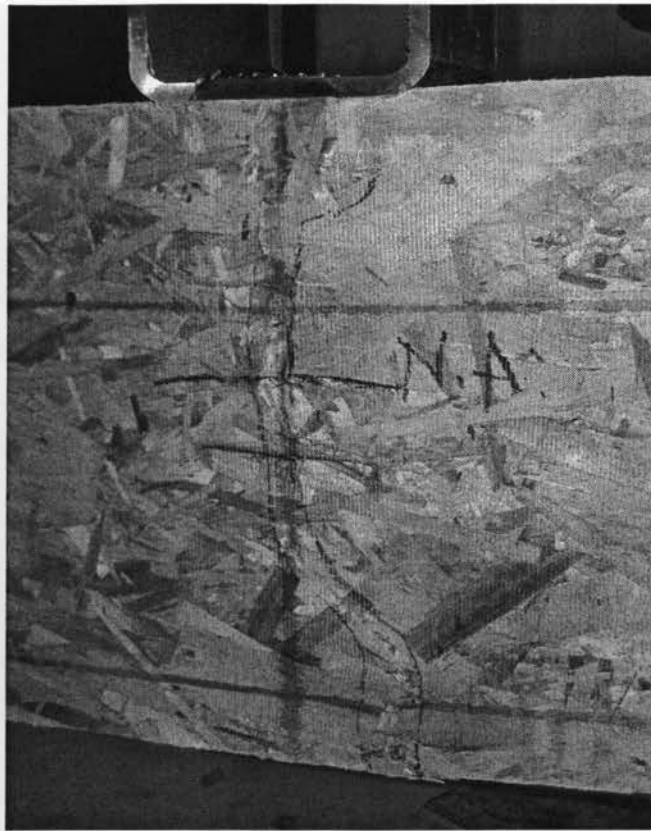
Figure 4.81 Neutral axis after the flexure failure mode of header H-15 at loading point
