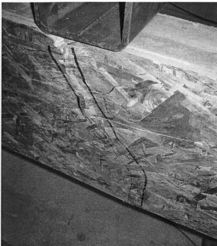
Figure 4.67 Close-up view of the flexure failure mode at quarter point of header H-13
