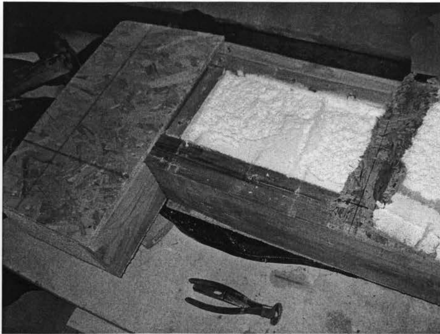
Figure 4.9 Close-up view of the foam and header end after removing the deformed OSB web of header H-2
