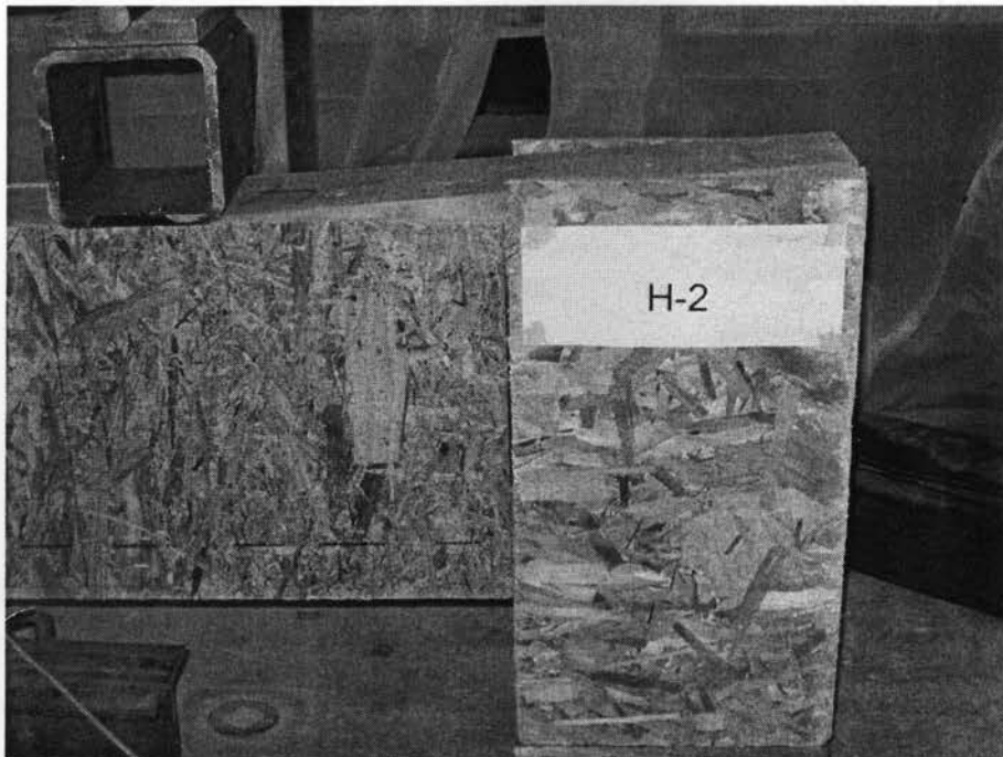
Figure 4.8 Close-up view of the failure mode of header H-2
