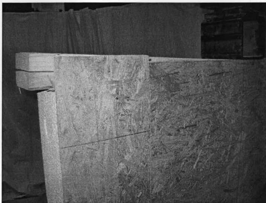
Figure 4.49 Close-up view of the failure mode of the left side of header H-10
