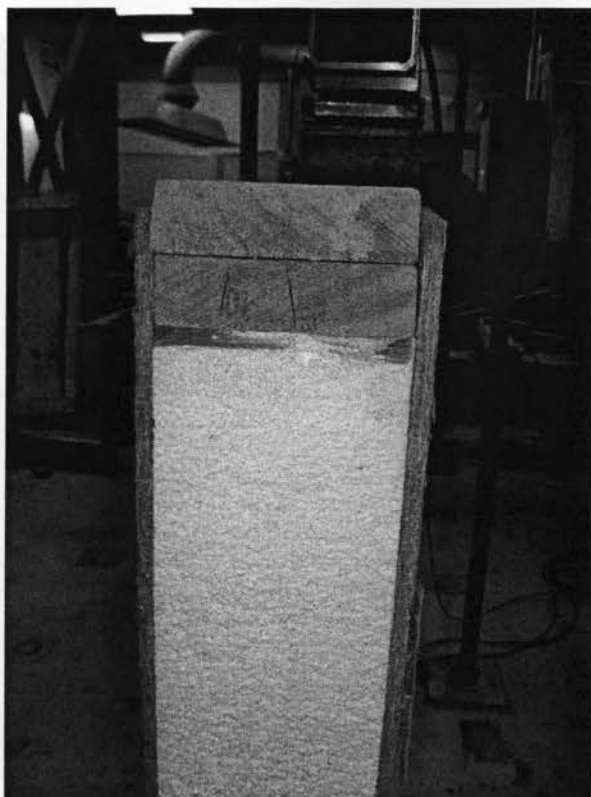
Figure 4.86 View of the foam at the location of failure of header H-16
