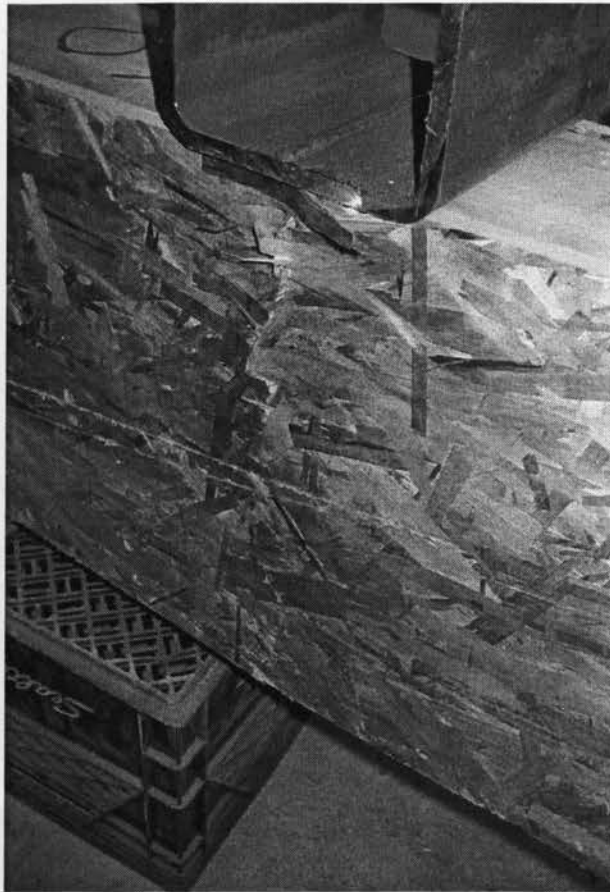
Figure 4.64 Close-up view of the flexure failure mode at quarter point of header H-13
