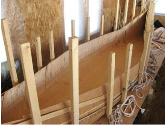
Figure 3.28 Canoe construction – structural supports
