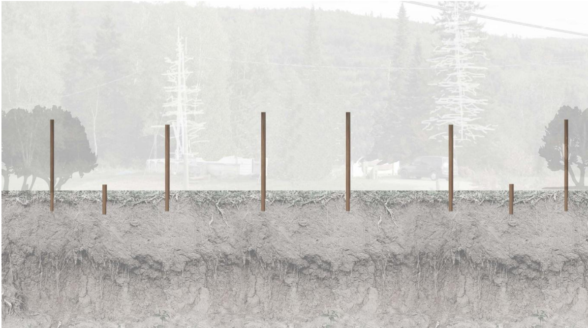
Figure 3.15 Site 2 – minimal intervention on land – pile foundation
