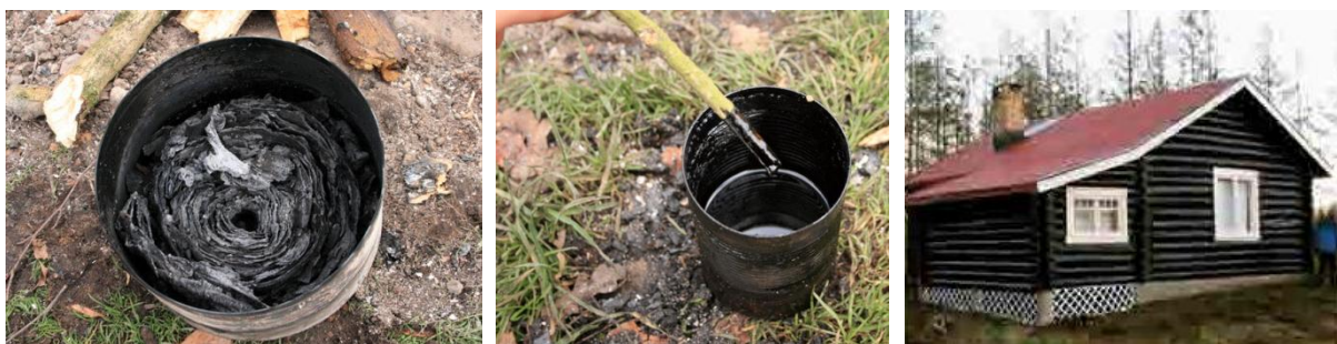
Figure 4.6 From left to right: Boiling Birch bark to form tar and wooden house in Scandinavia preserved through application of Birch tar. Image credit: Wingard
