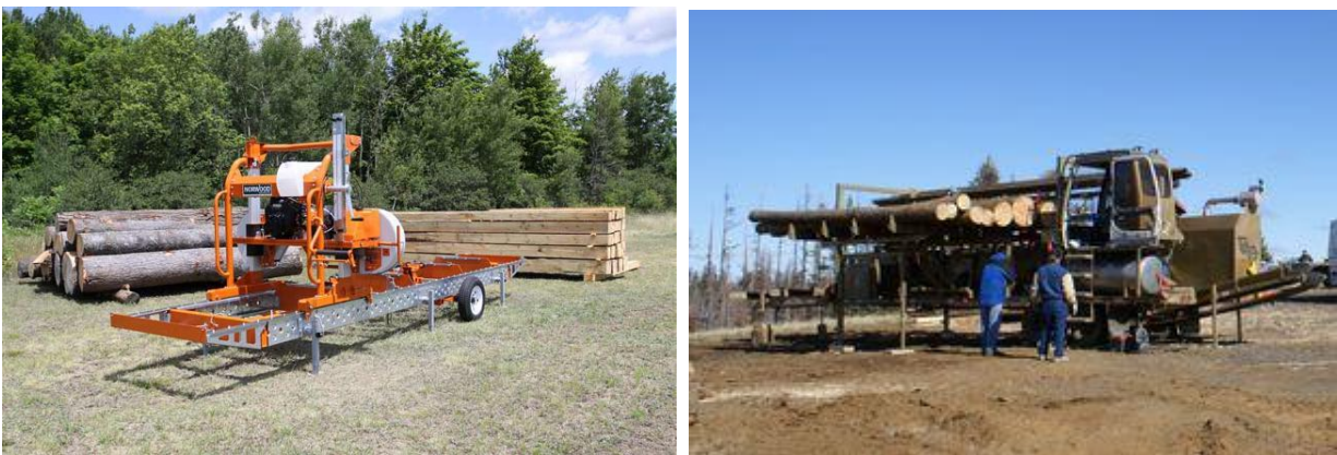
Figure A.6 Portable Sawmill ~$36,000 and Twin-cut Mobile Automated Sawmill ~$260,000 Image credit: Norwood Industries Inc. and DaveCo
