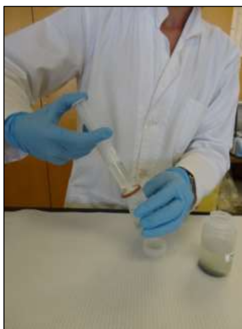
b. Separate Sorbate (HMI) and Sorbent (Zeolite) with Syringe-Filter
