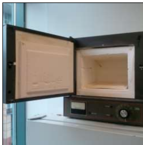
b. Place the Measured Zeolite Mass onto the Tray, then into the Muffle Furnace
