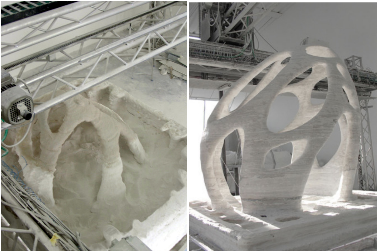
Figure 8.3.1 Printing of sandstone structure in one continuous session.
