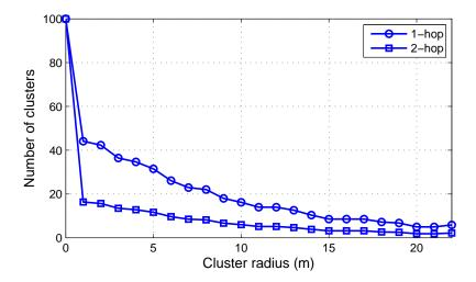
Figure 6.9: The minimal dominating set vs cluster radius for 1 and 2-hop clustering
