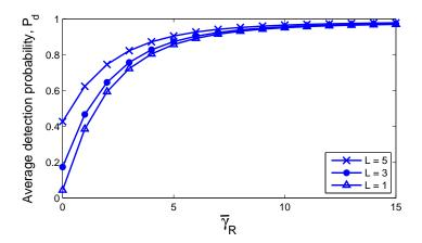
Figure 5.4: Average detection probability,  $\overline{P}_d$ , vs.  $\overline{\gamma}_r$ , for L=1, 3, and 5.  $\overline{\gamma}_s = 5 dB$ , u = 8.
