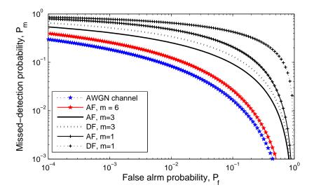
Figure 3.4: Complementary ROC curves at different relaying channel conditions. P=5 dB,  $L=3, \, \overline{\gamma}_s=0$  dB.
