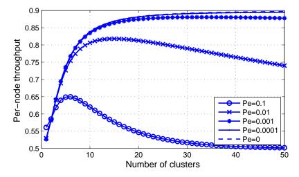
Figure 6.7: The normalized per-node throughput vs number of cooperative clusters,  $u = 12, \, \overline{\gamma}_s = 10 \text{ dB}$
