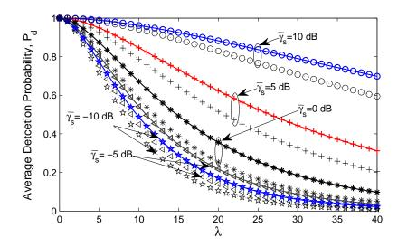
Figure 3.5: Average detection probability for different level of sensing channel SNR. P = 5 dB, L = 3, m = 2.
