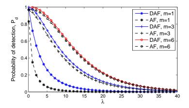
Figure 4.4: Detection performance of AF and DAF strategies for different fading scenarios with L = 3, P = 5 dB, and  $\overline{\gamma}_s = 0$  dB.
