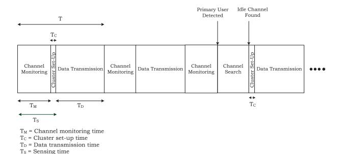
Figure 2.4: Sensing round structure in cluster-based spectrum sensing
