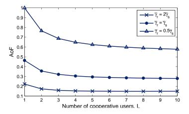
Figure 5.5: Amount of fading vs. number of cooperative users.  $\overline{\gamma}_s = 10 \ dB$ .
