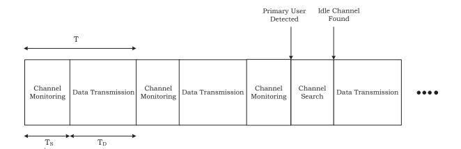
$T_M$  = Channel monitoring time  $T_D$  = Data transmission time  $T_S$  = Sensing time T = Sensing period (frame size)
