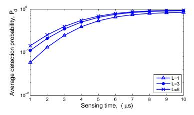
Figure 5.3: Average detection probability  $\overline{P}_d$  vs. sensing Time for L=1, 3, and 5.  $\overline{\gamma}_s = \overline{\gamma}_r = 5 \ dB$ .
