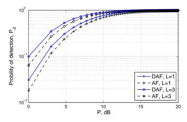
Figure 4.5: Detection performance of AF and DAF strategies for different power constraints with  $\lambda = 5$ , m=2, and  $\overline{\gamma}_s = 0$  dB.
