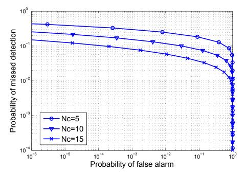
Figure 6.5: Cluster-based cooperative sensing performance with various cluster size, u = 12,  $\overline{\gamma}_s = 10$  dB
