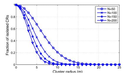
Figure 6.4: Fraction of single-node clusters vs cluster radius under different node densities
