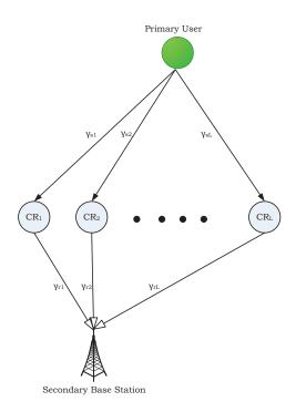
Figure 2.1: Centralized cooperative spectrum sensing system.
