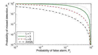
Figure 4.2: ROC curves of the energy detector with m=2, P=5 dB, and  $\overline{\gamma}_s=0$  dB.
