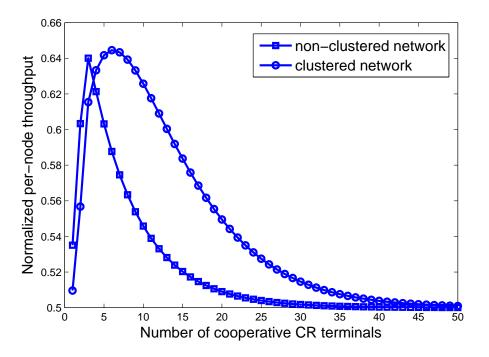
Figure 6.8: Per-node throughput performance of clustered and non-clustered network vs number of cooperative terminals, u = 12,  $\overline{\gamma}_s = 10$  dB
