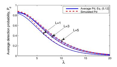
Figure 5.1: Comparison of average detection probability in equation (5.12) with Monte Carlo simulation for L=1, 2, and 3.  $\overline{\gamma}_s = \overline{\gamma}_r = 5 \ dB, \ u = 6.$
