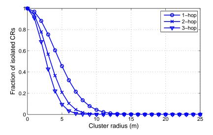
Figure 6.3: fraction of single-node clusters vs cluster radius for 1, 2, 3-hop clusters
