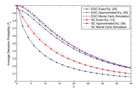
Figure 3.3: Comparison of analytical and simulated  $\overline{P}_d$ . P = 5 dB, L = 3, m = 2,  $\overline{\gamma}_s = 0$  dB.
