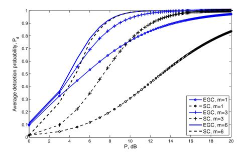
Figure 3.6: Average detection probability vs. relay maximum transmitting power, P.  $L=3,\,\lambda=20,\,\overline{\gamma}_s=0~{\rm dB}$
