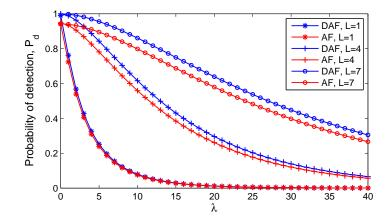
Figure 4.3: Detection performance of AF and DAF strategies for different diversity scenarios with m = 2, P = 5 dB, and  $\overline{\gamma}_s = 0$  dB.
