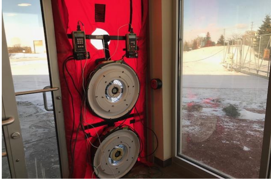
Figure 8: Air-leakage test (blower door test)
