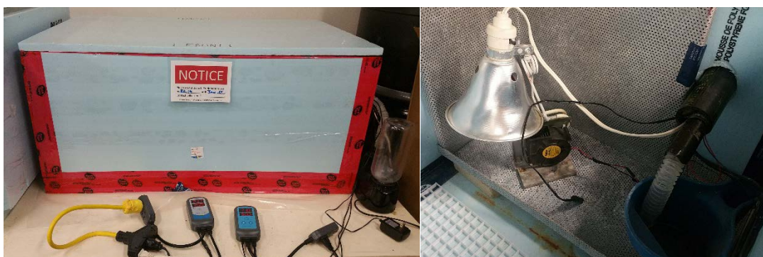
Photograph 3.5 - Environmental Chamber Used to Condition Thermal Conductivity Specimens.
