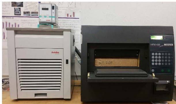
Photograph 3.6 - Heat Flow Meter Apparatus with Specimen.
