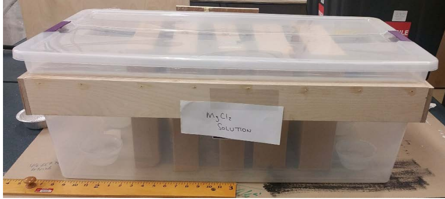
Photograph 3.7 – Salt Solution Environmental Chamber Used to Condition Thermal Conductivity Specimens.
