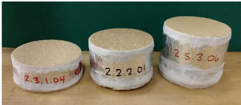
Photograph 3.2: Vapour Permeance Specimens with Edge Masking.
