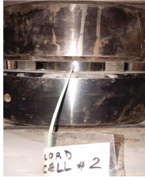
Figure 3.16: Load cells and steel covers.
