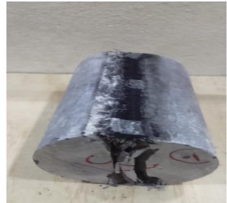
Figure 3.12: Cylindrical specimens after indirect tensile strength test.
