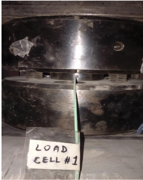
Figure 3.16: Load cells and steel covers.
