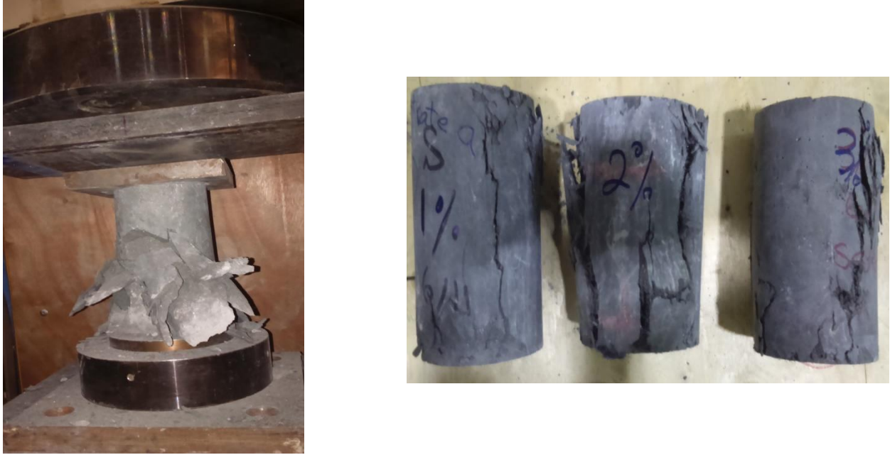
Figure 3.9: Cylindrical specimens after compressive strength test.
