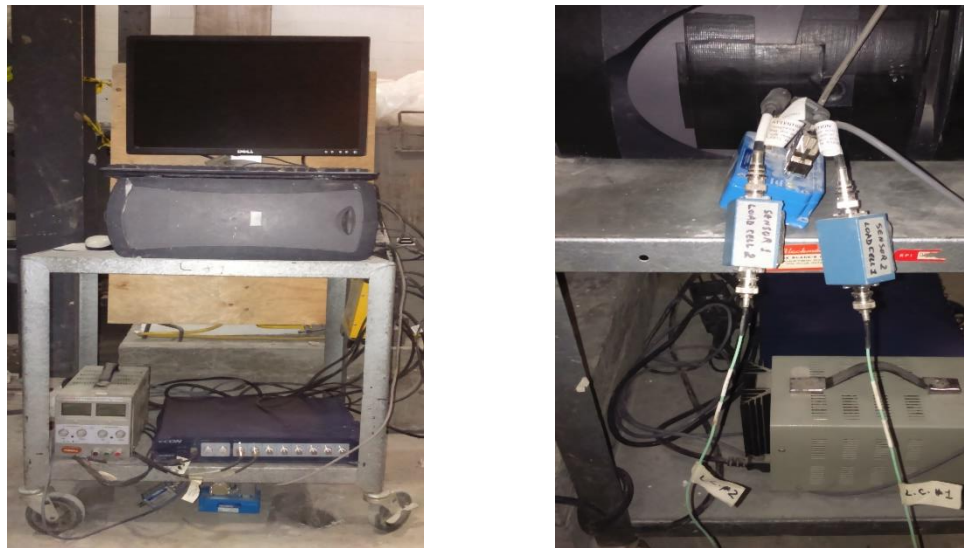
Figure 3.19: Data acquisition system, computer, and connections.
