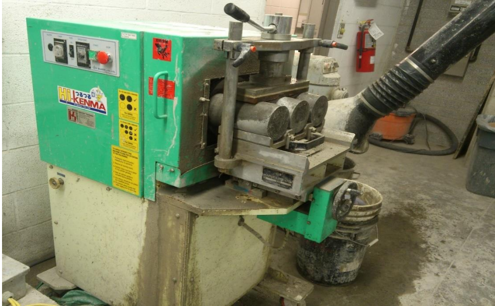
Figure 3.6: Concrete cylinder end grinding machine.
