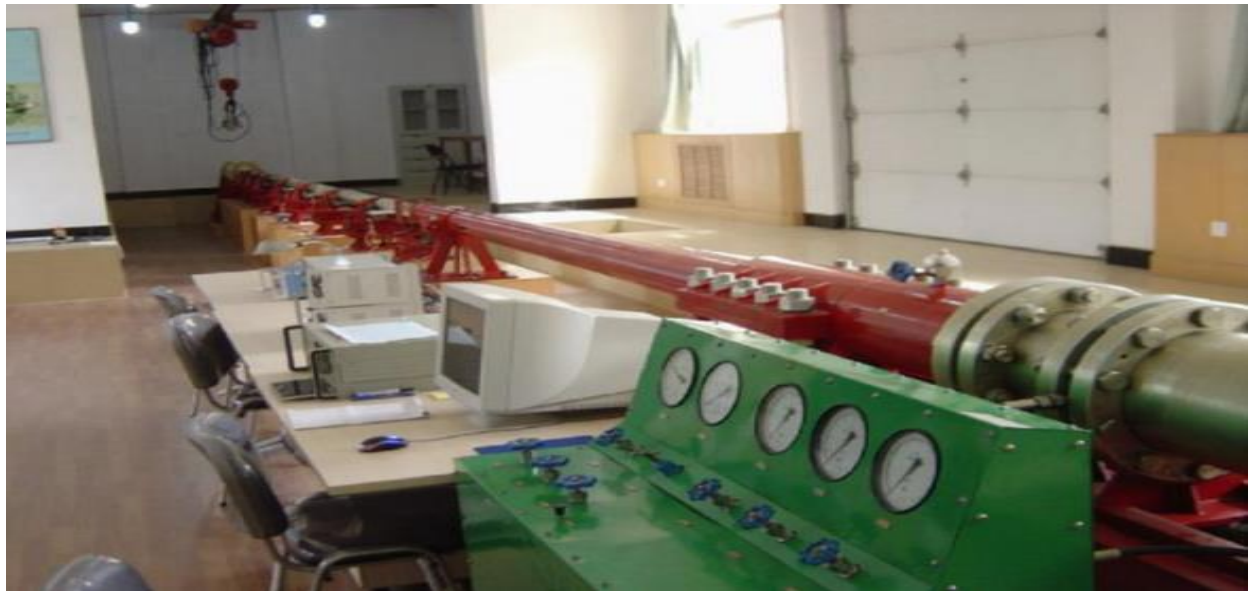
Figure 2.8: SHPB setup for testing concrete specimens under compression [66].
