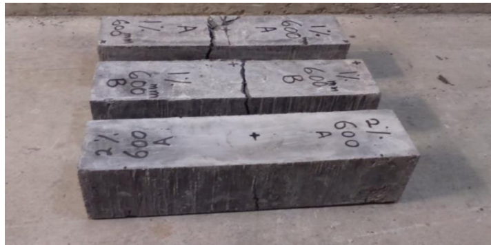
Figure 4.5: UHP-FRC specimens with 1 & 2% fiber, after impact test (drop height: 600 mm).
