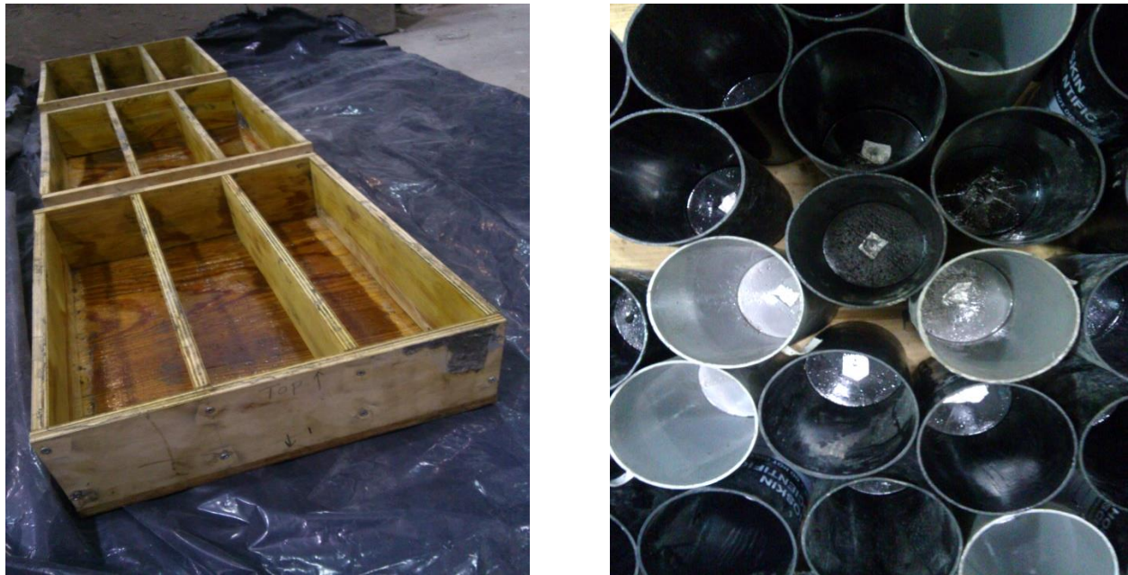
Figure 3.4: Prism and cylinder molds before casting.
