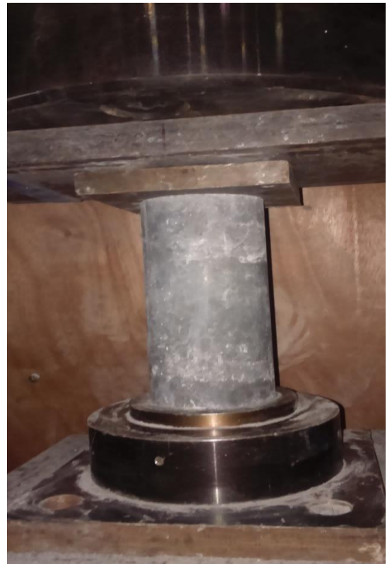
Figure 3.8: MTS 815 test system – Compressive strength test.
