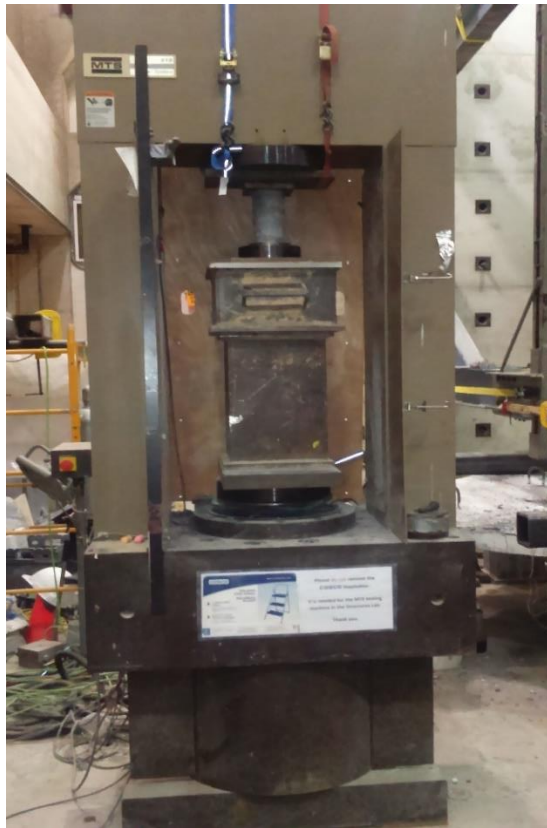
Figure 3.8: MTS 815 test system – Compressive strength test.
