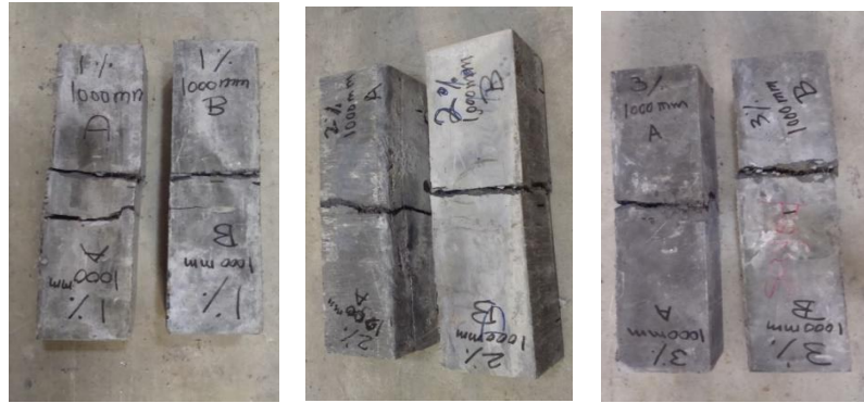
Figure 4.6: UHP-FRC specimens with 1, 2 & 3% fiber, after impact test (drop height: 1 m).
