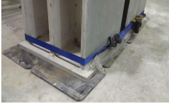
Figure 3.20: Steel pedestals rested on rubber pads.
