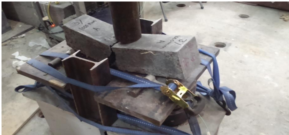
Figure 4.4: A UHP-FRC prism specimen after impact test.
