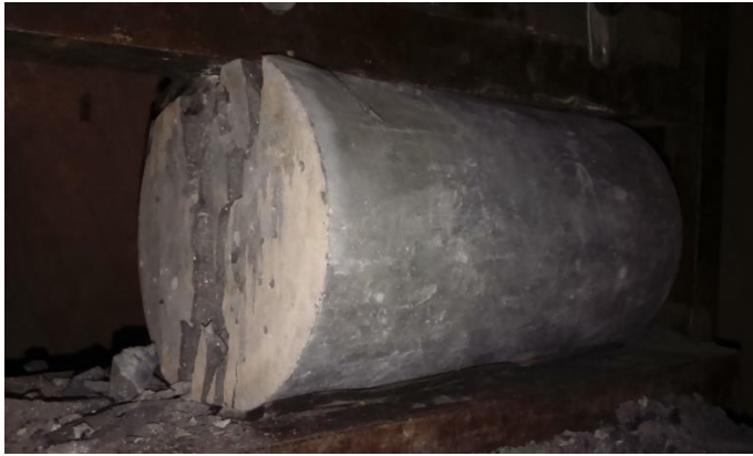
Figure 3.12: Cylindrical specimens after indirect tensile strength test.
