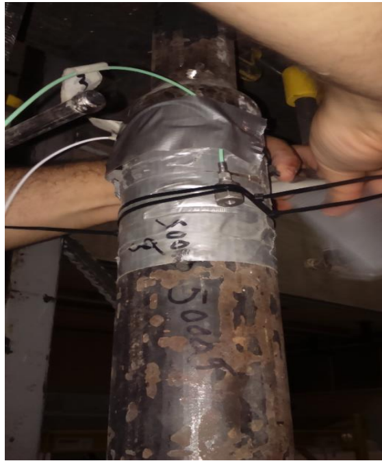
Figure 3.18: installation of the accelerometers on the drop weight.
