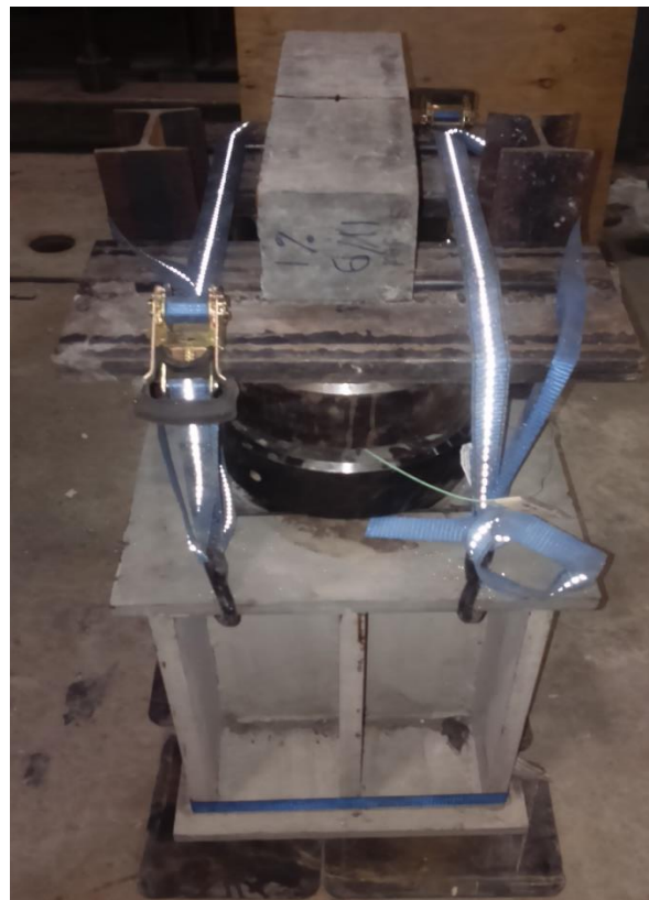
Figure 3.17: Prism specimen before conducting impact test.
