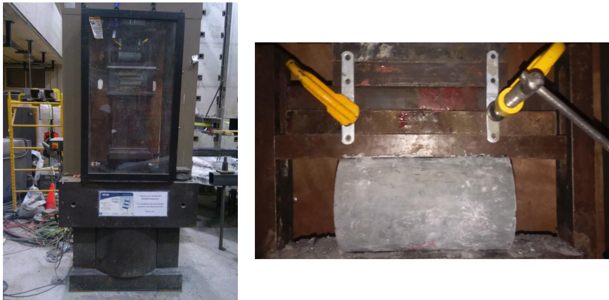
Figure 3.11: MTS 815 test system – Indirect tensile strength test.
