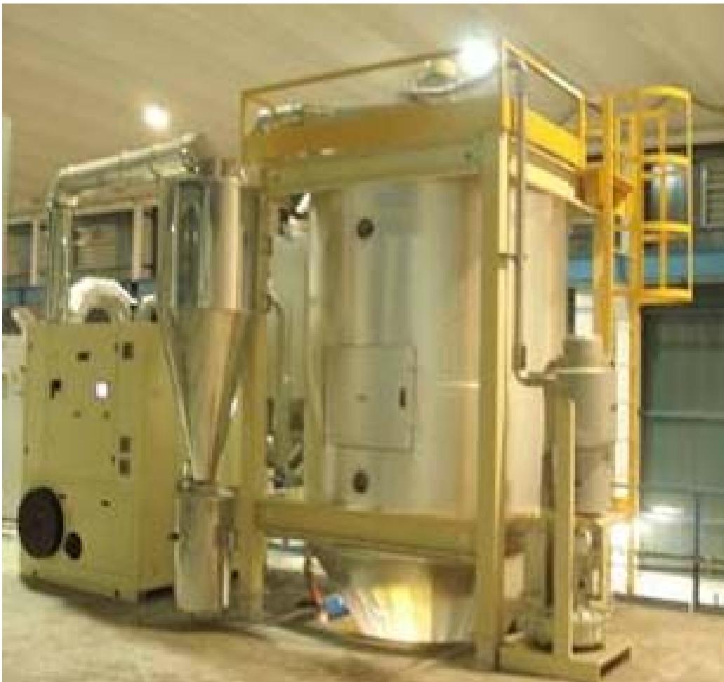
Figure 9: The Piovan resin dryer (3500 Liter DP628L) utilized in the validation test
