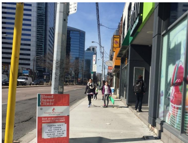
Figure 5-9: Insufficient Sidewalk Clear zone at Yonge St East side
