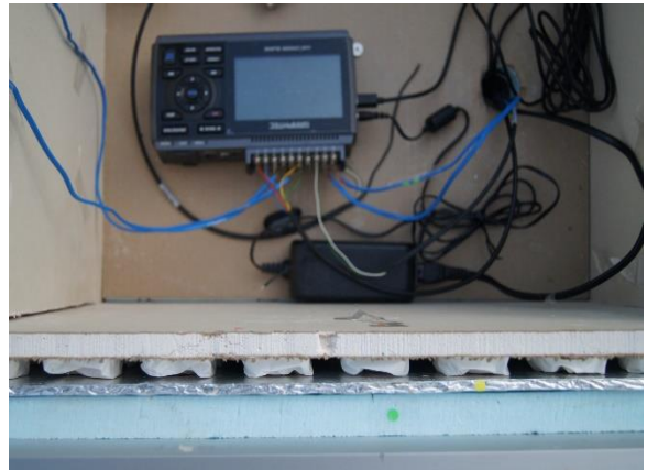
2) Wall assembly configurations (Left) – Connection of sensors to the data logger (Right)
