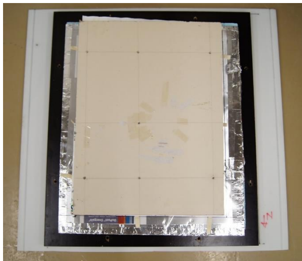
1) Ceiling structure of the composite PCM test cell
