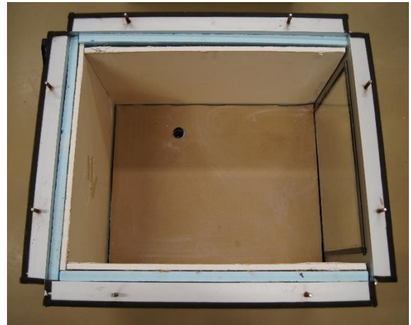
3) The composite PCM test cell (Left)- Reference test cell (Right)
