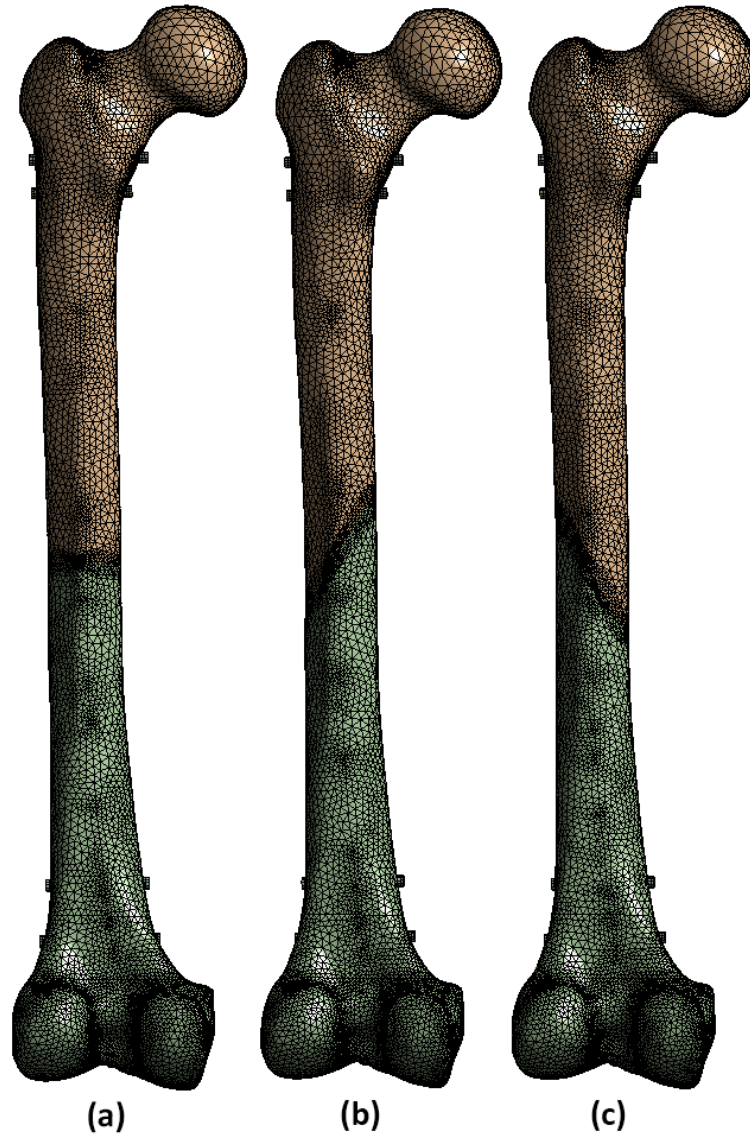
Figure 6-1. Finite element models of a femur with a transverse (a), proximal medial to distal lateral (PMDL) oblique (b), and proximal lateral to distal medial (PLDM) oblique (c) fracture, which was fixed with an IM nail.
