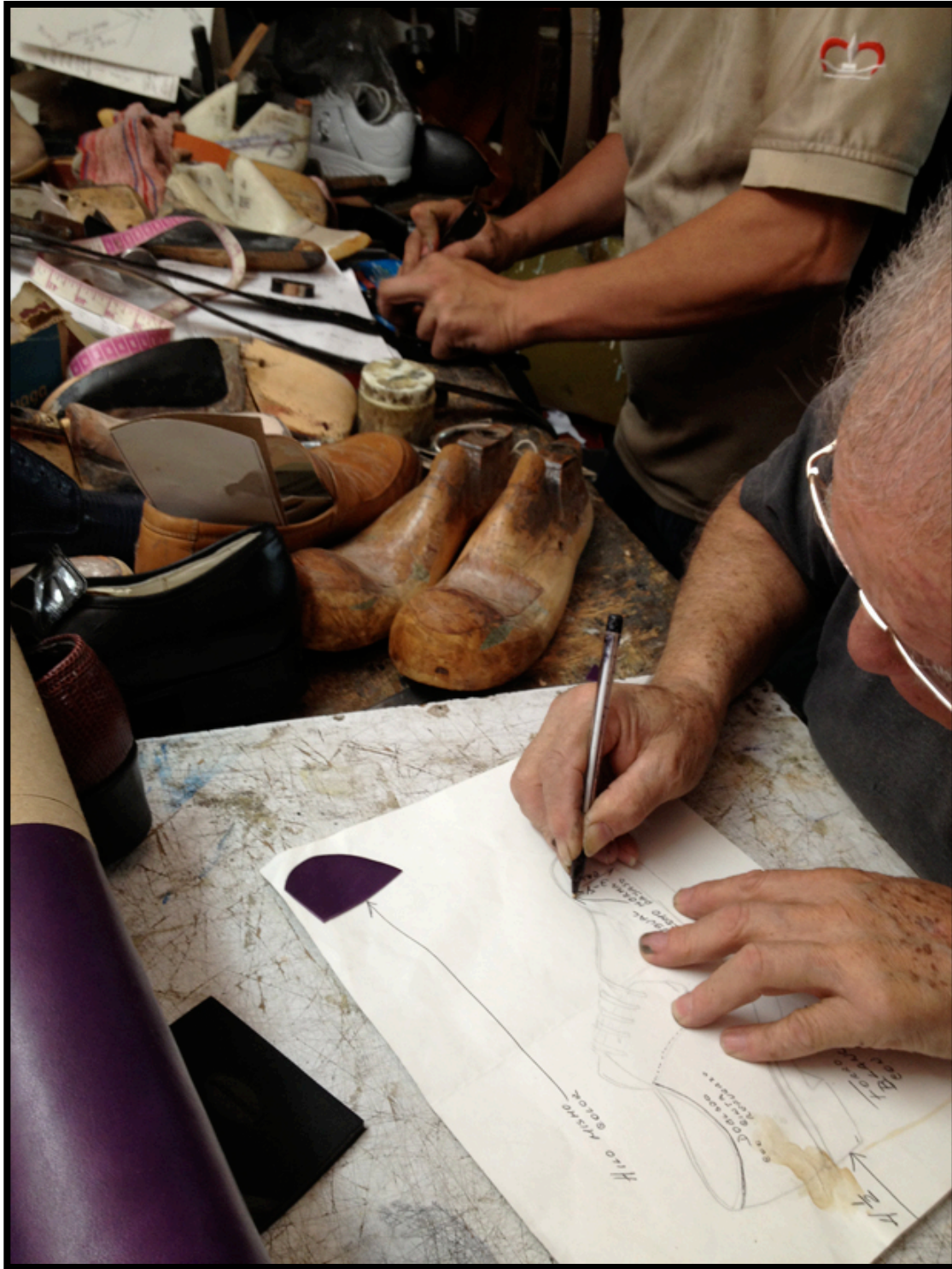
Figure 19. Photograph of The CLOWN derby design details. Technical spec sheet and lasts.
