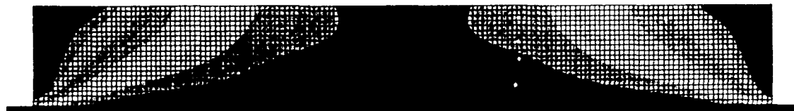
Figure A.1.12: Contour plot of longitudinal steel strains ( L = 30m , H = 4m , t = 300mm , \rho = 0.5\% , \varepsilon = 150 \times 10^{-6} ), development of cracks with increasing volumetric deformation
