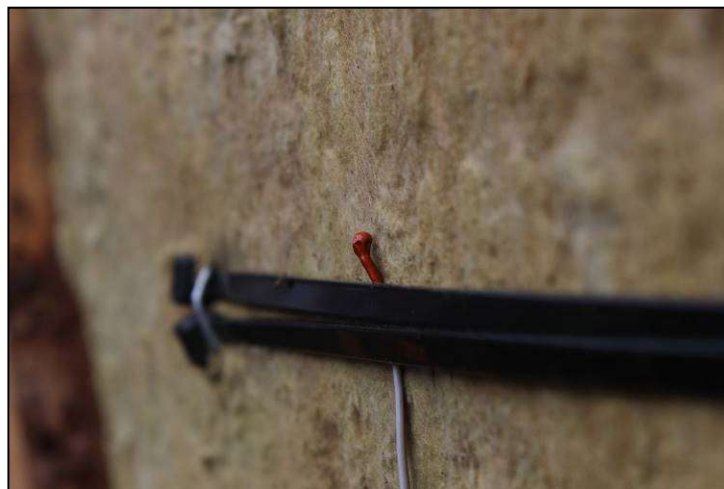
Figure 4-5 : Temperature Sensor - Layer 2
