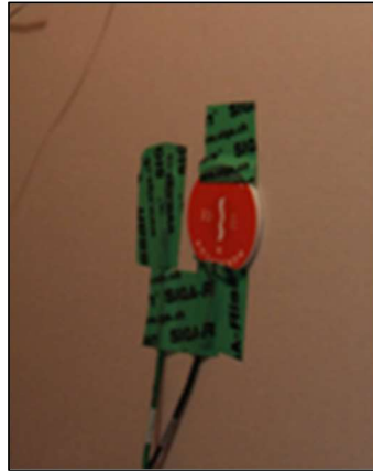
Figure 3-11 : HFP01 Plate and Thermocouple
