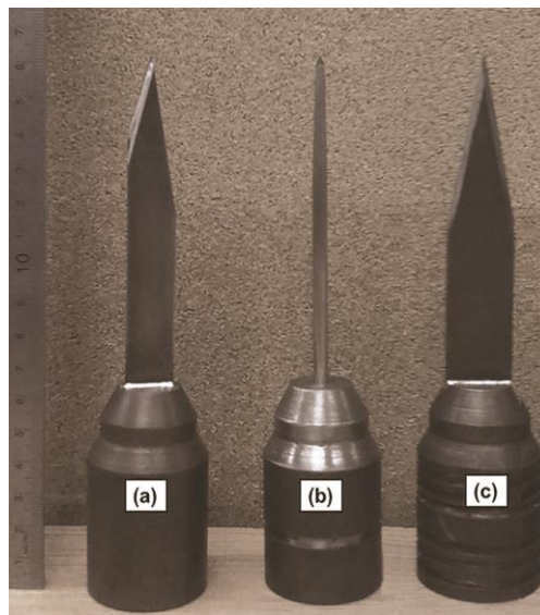
Figure 12. Weapons used for the penetration test on fabrics according to the NIJ Standard 0115.00 [116]: (a) P1 blade, (b) Spike, and (c) S1 blade.
