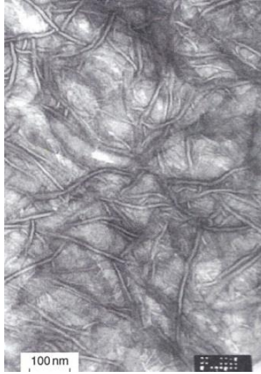
Figure 4. A TEM image of UHMWPE showing amorphous (gray color) and crystalline regions (white lines with a dark out-line) [43].
