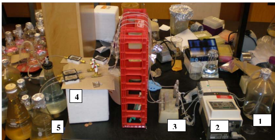
Figure 4. Experimental Set-up. a) Simplified schematic and b) photograph, of experimental set-up 1) medium reservoir, 2) peristaltic pump, 3) bubble trap, 4), Flow cell containing the rock wafer, 5) effluent. Silicon tubing was used to the right of the tee junction. Teflon tubing was used to the left of the tee junction – seen between 3 and 4 - in b.
