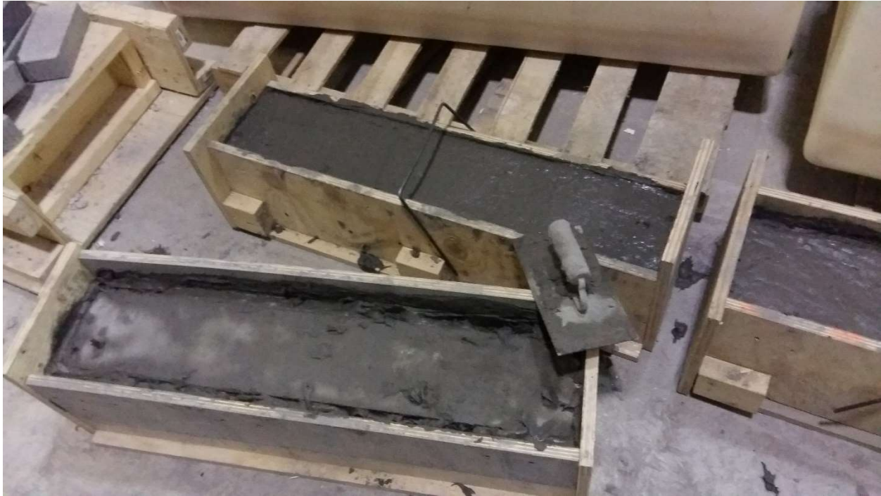
Fig. 3.4: Casting of ECC wrapping around core columns
