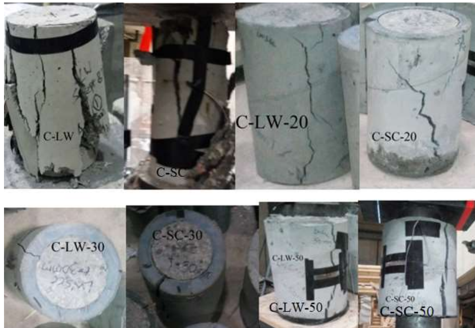
Fig. 4.4: Testing of cylindrical columns showing crack patterns and failure modes
