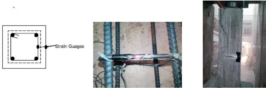
Fig. 3.13: Location of strain gauge for columns and testing
