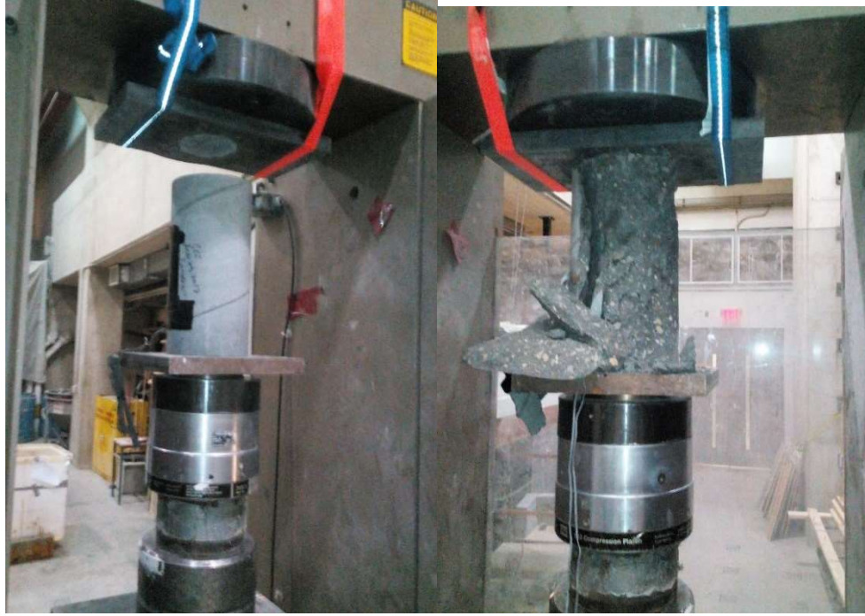
Fig. 3.5: Experimental set-up, instrumentation, and testing of concrete cylinders
