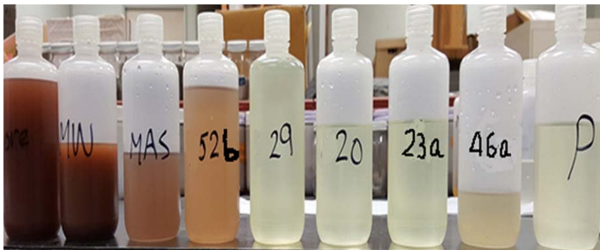
Figure 3 - 7: The colour of sodium hypochlorite solution after the first cycle (two-weeks) of the test.
