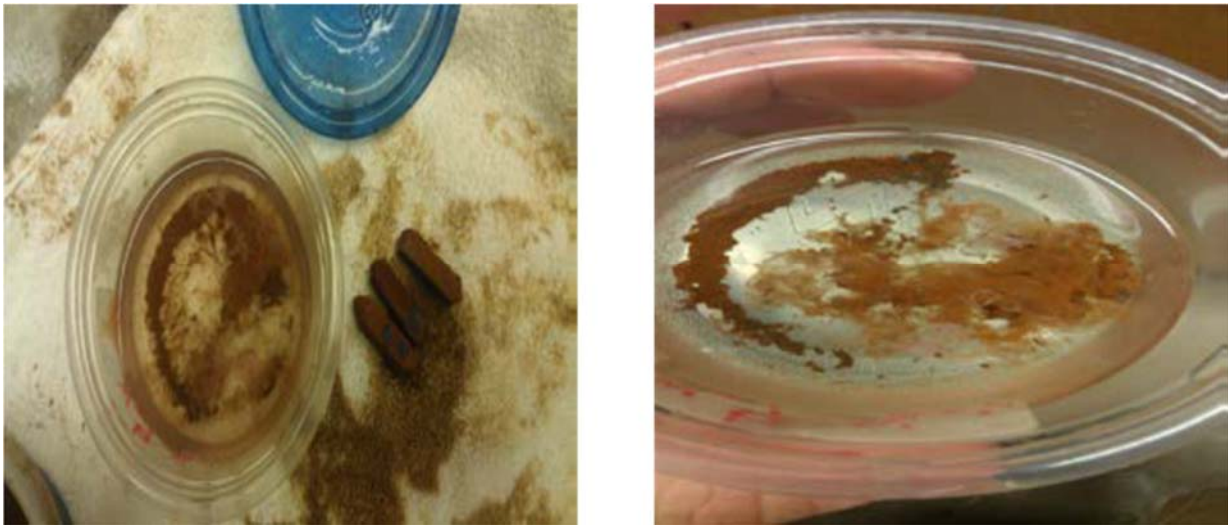
Figure 3 - 4: MW oxidized samples and some iron oxide precipitated onto the container
