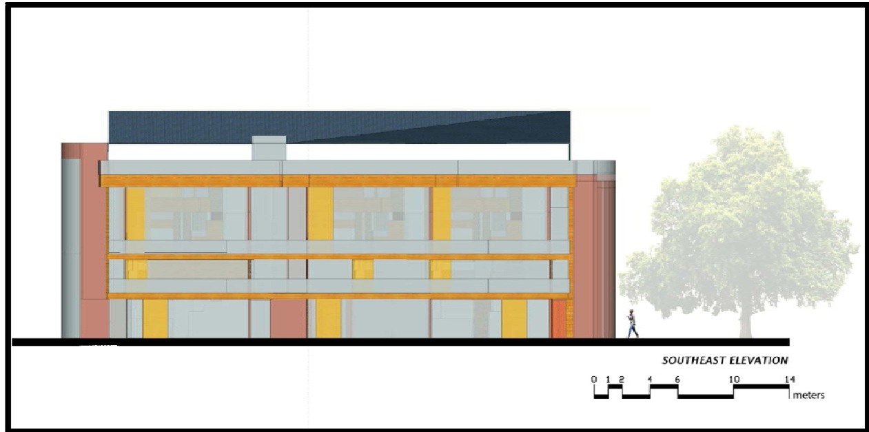
Figure 4.22: The elevation shows the moveable vertical wooden panels against the west sun.
